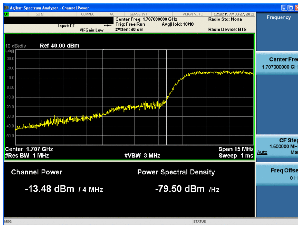
Plot 7-3. Lower Extended Band Edge Plot (5MHz QPSK- RB Size 25)
