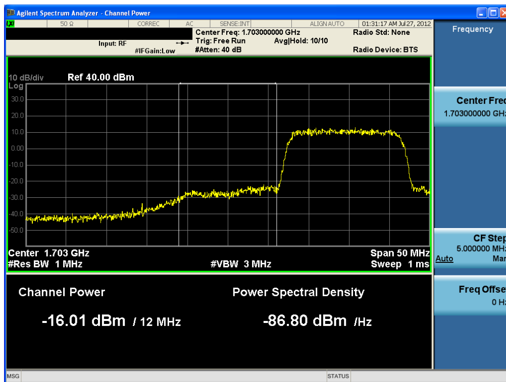
Plot 7-17. Lower Extended Band Edge Plot (QPSK – RB Size 75)
