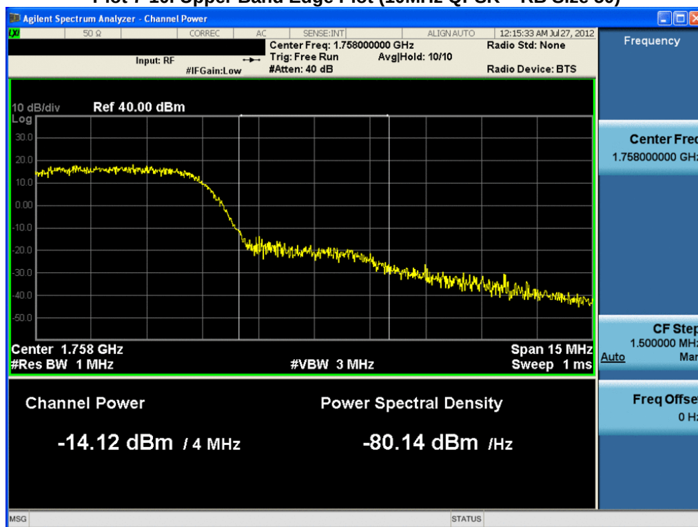
Plot 7-11. Upper Extended Band Edge Plot (5MHz QPSK– RB Size 25)
