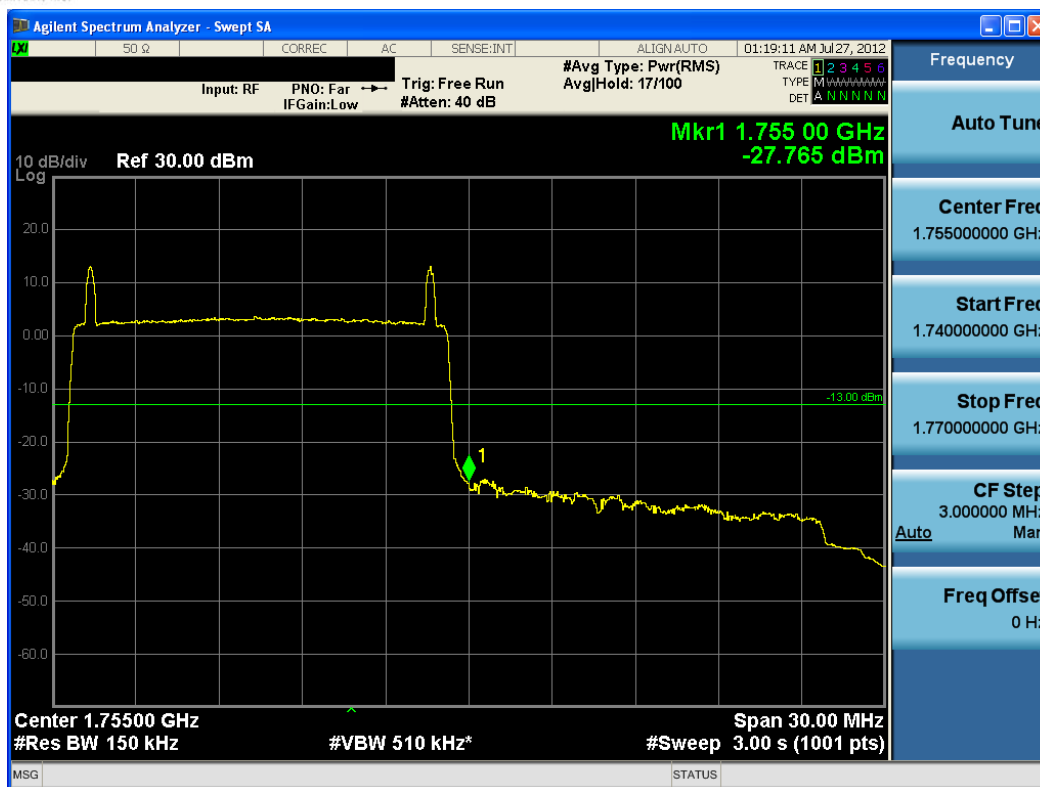
Plot 7-29. Upper Band Edge Plot (QPSK – RB Size 75)
