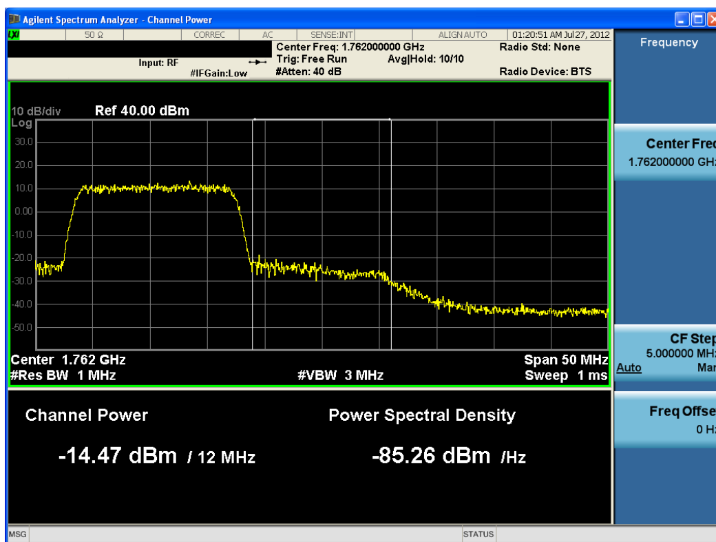
Plot 7-30. Upper Extended Band Edge Plot (QPSK – RB Size 75)
