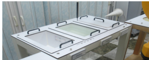
Figure 3.6 Modular Flat Phantom
