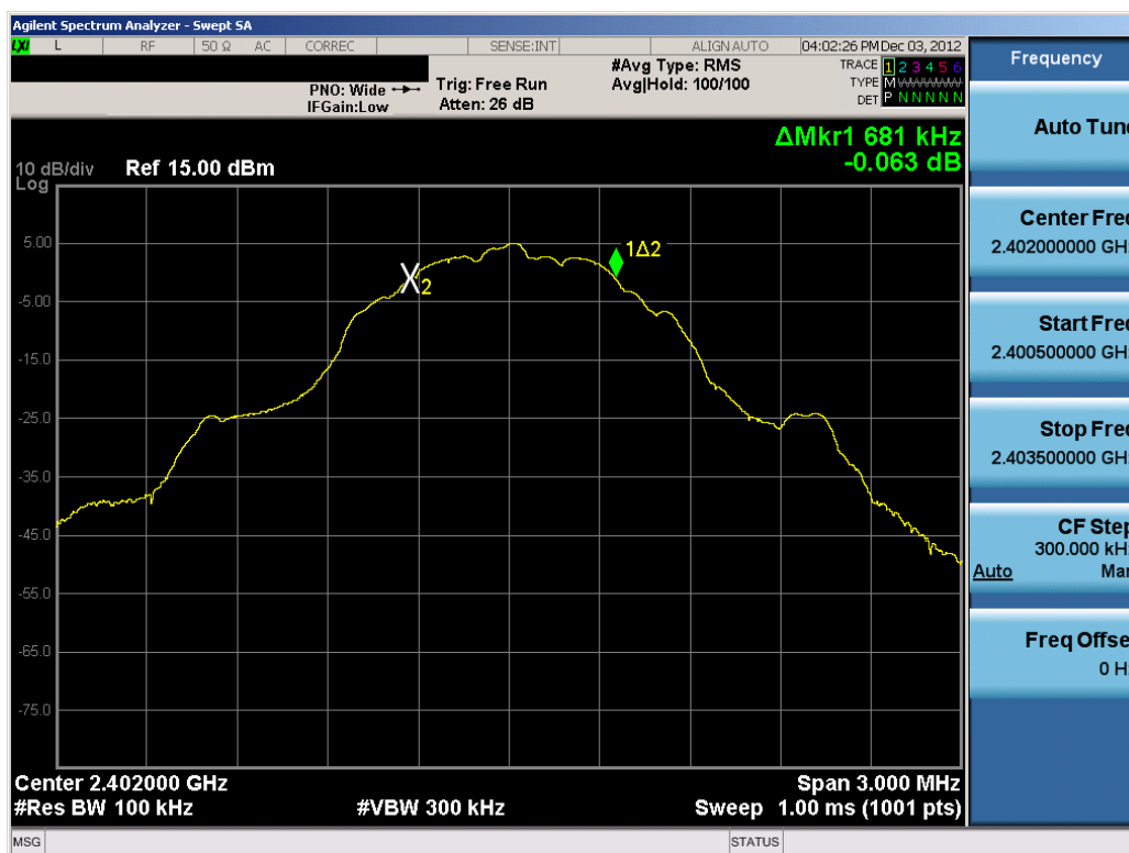
Plot 6-1. 6dB Bandwidth Plot (Bluetooth (LE) – Ch. 0)
