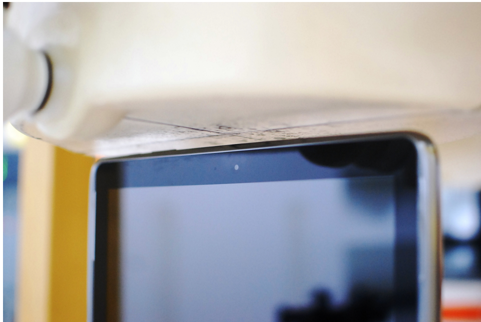
SAR Test Setup Photo 4 – Top Edge at 1.0 cm
