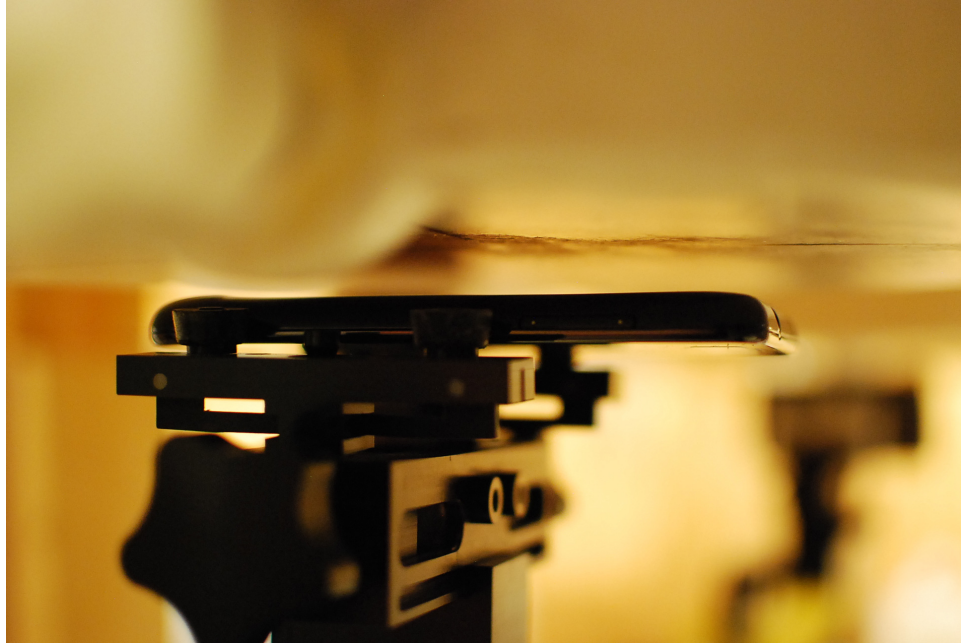
SAR Test Setup Photo 5: Back at 1.0 cm
