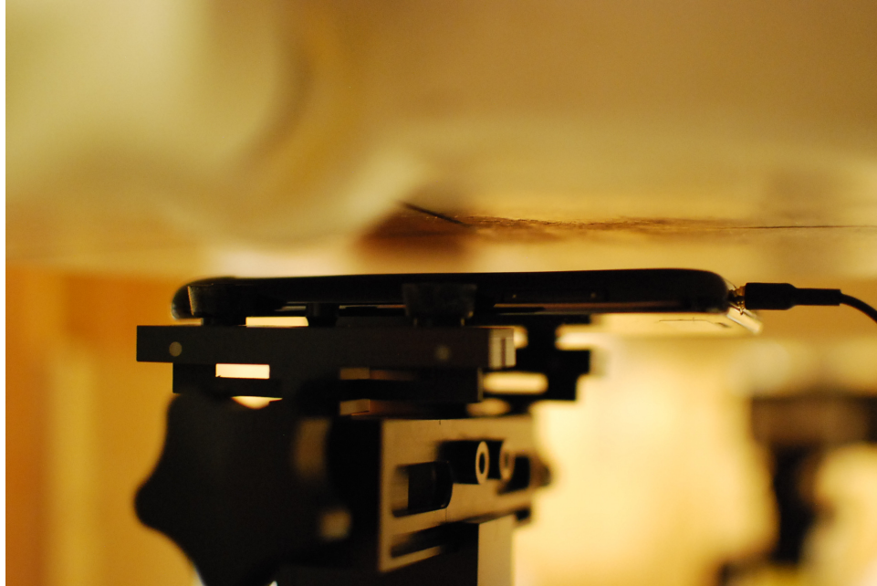
SAR Test Setup Photo 11: Body-Worn at 1.0 cm
