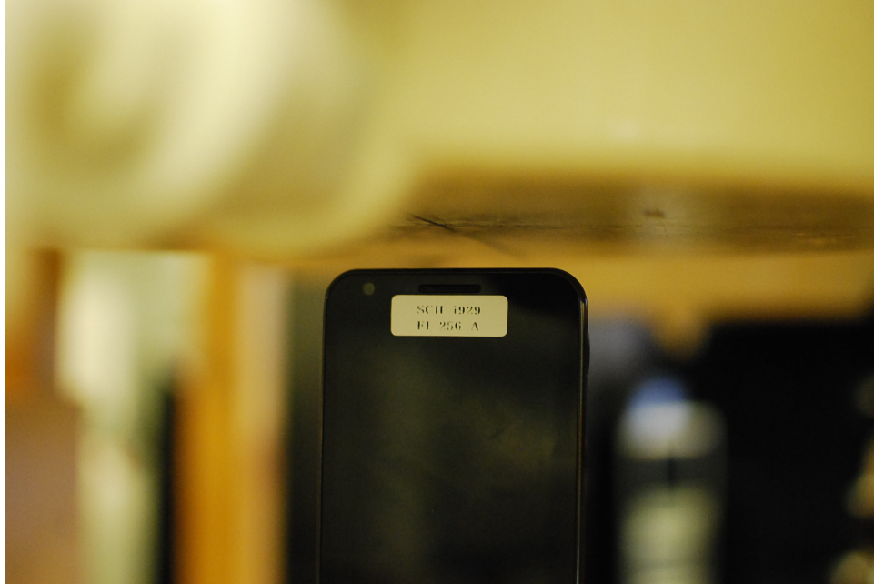
SAR Test Setup Photo 7: Top at 1.0 cm
