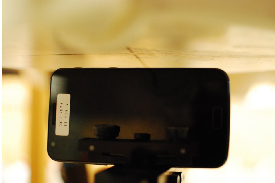
SAR Test Setup Photo 9: Right at 1.0 cm
