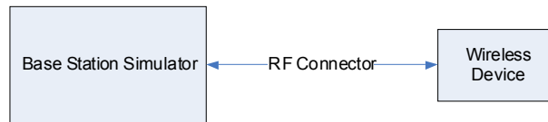
Figure 10-3 Power Measurement Setup
