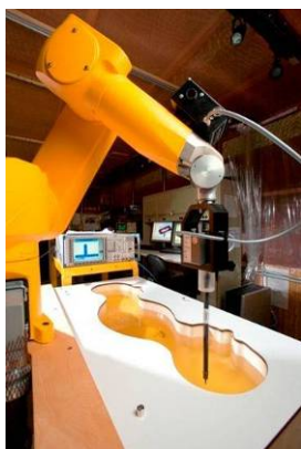
Figure 4-1 SAR Measurement System
