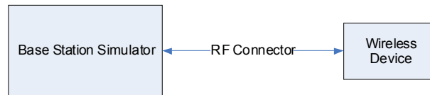
Figure 10-3 Power Measurement Setup
