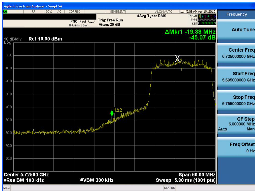
Plot 6-43. Band Edge Plot (802.11n (5.8GHz – 20MHz) – Ch. 149)
