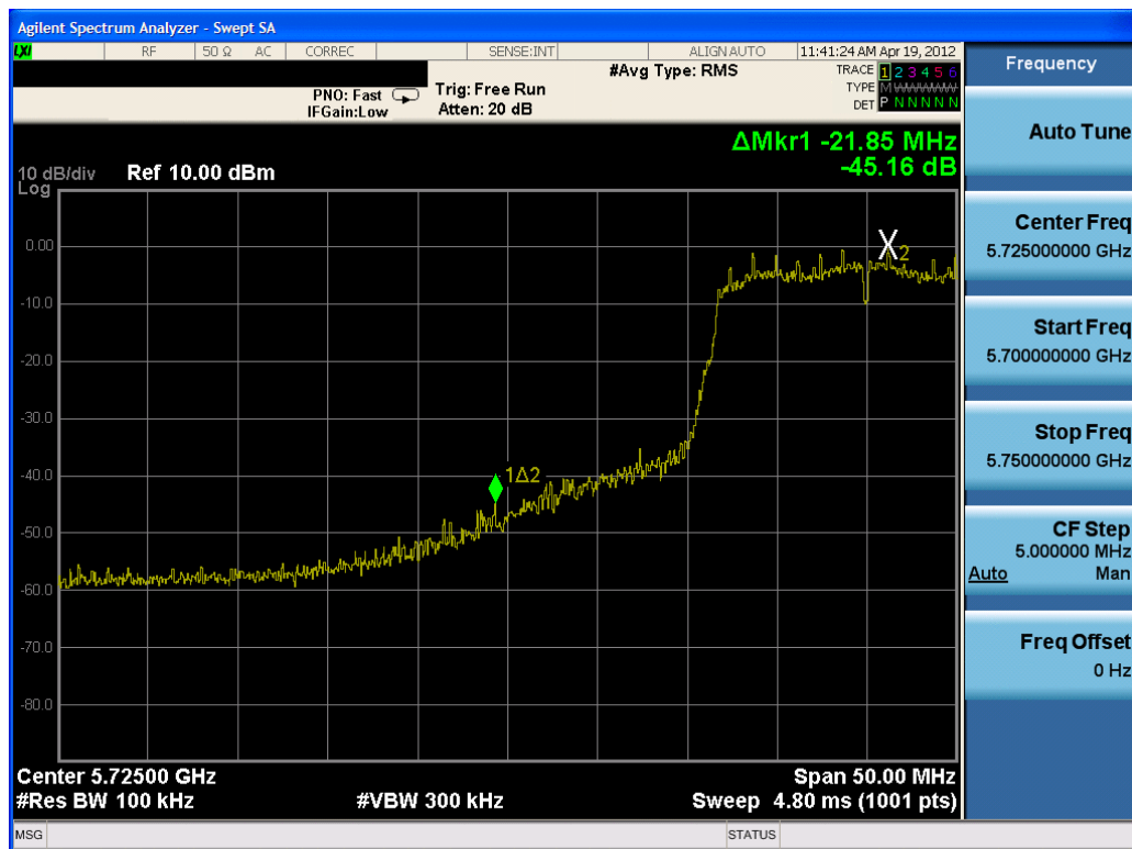
Plot 6-41. Band Edge Plot (802.11a – Ch. 149)
