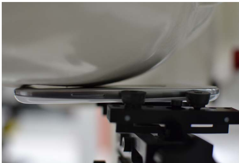
SAR Test Setup Photo 1 – Right Touch
