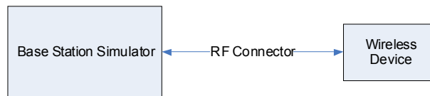
Figure 8-2 Power Measurement Setup
