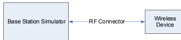
Figure 8-1 Power Measurement Setup
