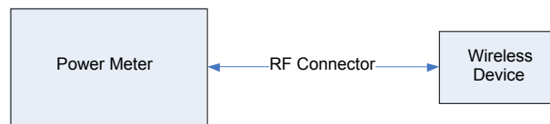
Figure 8-3 Power Measurement Setup
