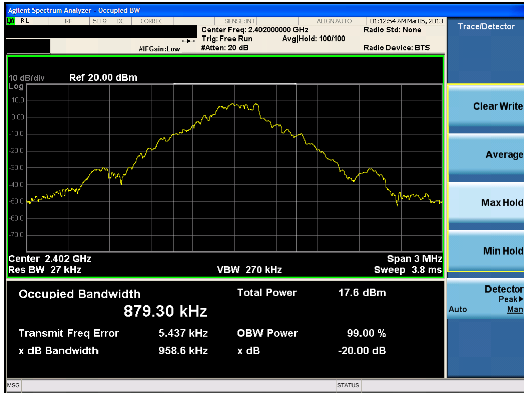
Plot 6-1. 20dB Bandwidth Plot (Bluetooth, 1Mbps – Ch. 0)
