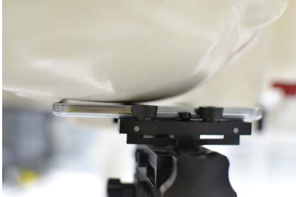
SAR Test Setup Photo 1 – Right Cheek
