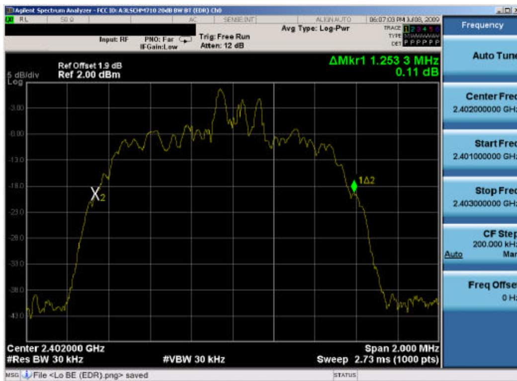
Plot 6-1. 20dB Bandwidth Plot (Bluetooth 2.1 with Enhanced Data Rates – Ch. 0)
