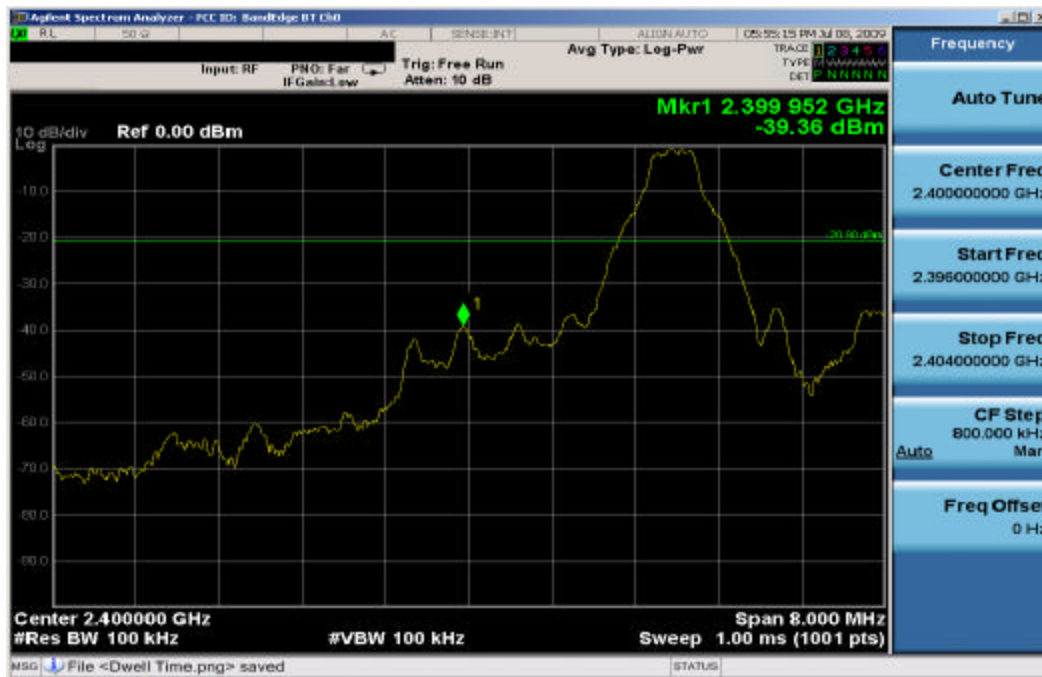
Plot 6-4. Band Edge Plot (Bluetooth – Ch. 0)
