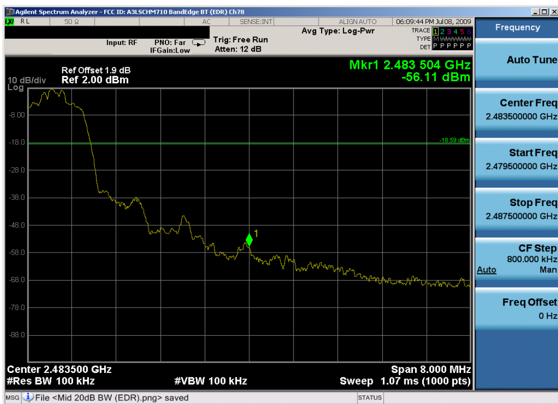
Plot 6-7. Band Edge Plot (Bluetooth 2.1 with Enhanced Data Rates – Ch. 78)
