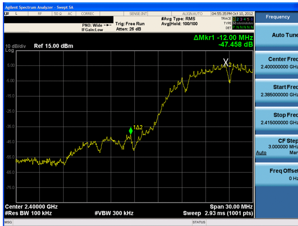
Plot 6-35. Band Edge Plot (802.11b – Ch. 1)
