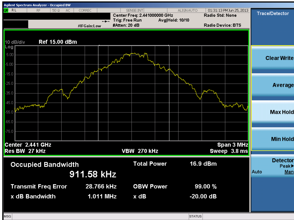
Plot 6-2. 20dB Bandwidth Plot (Bluetooth, 1Mbps – Ch. 39)
