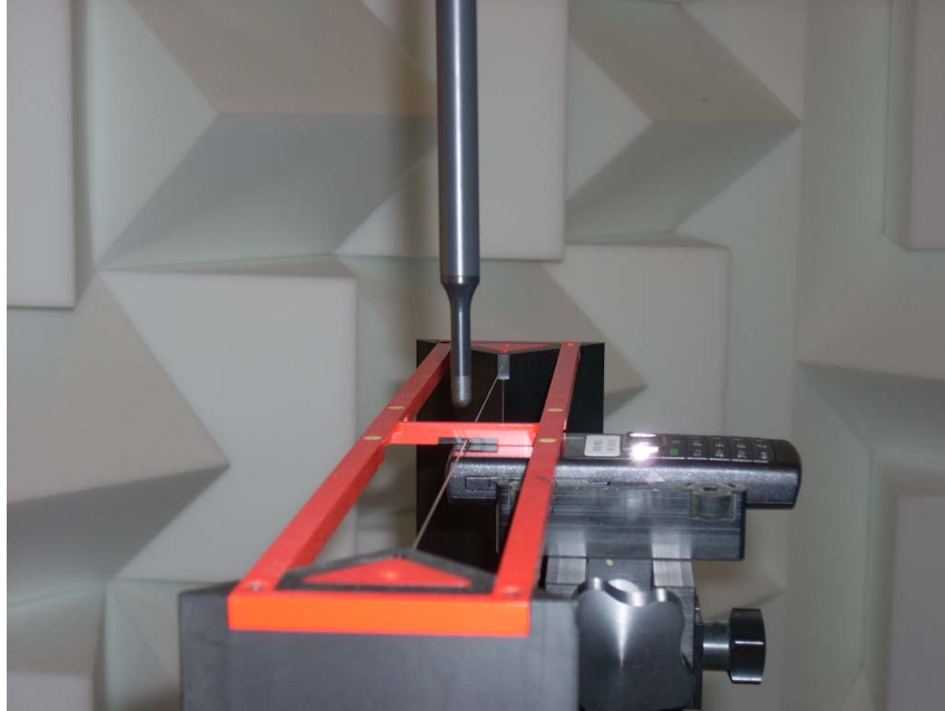
Figure 17-1 Ear Reference Point HAC Phantom Alignment
