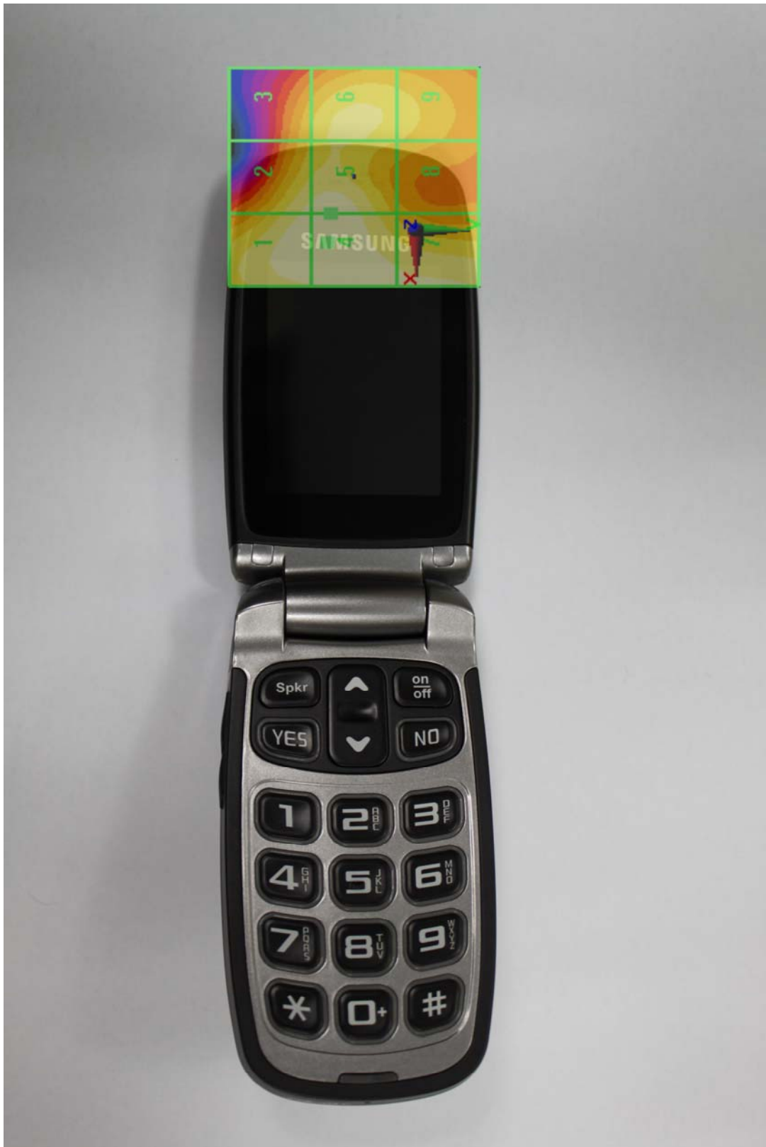
Scan Overlay with actual device(E-Field)
