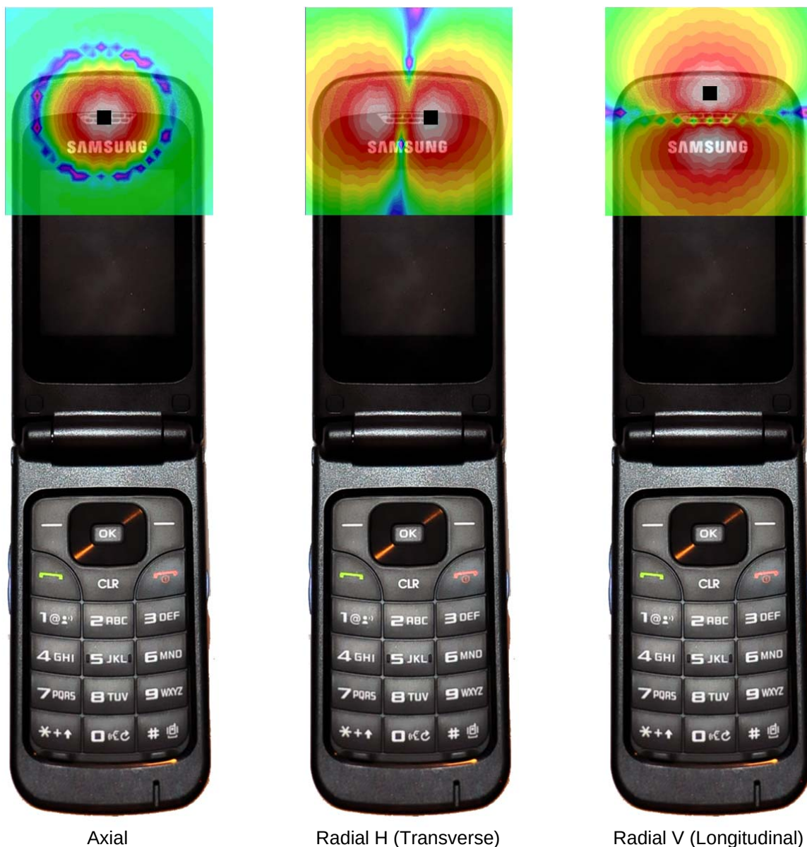
Figure 13-3 T-Coil Scan Overlay Magnetic Field Distributions
