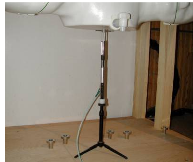
Figure 12-2 System Verification Setup Photo
