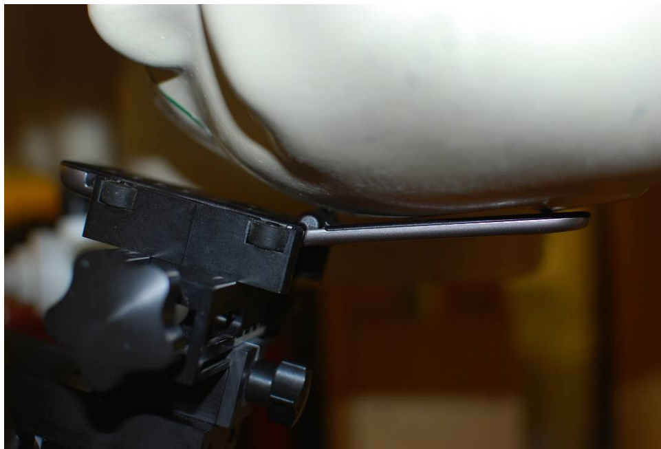
Figure 19-4 SAR Test Setup Photo 4 – Left Touch
