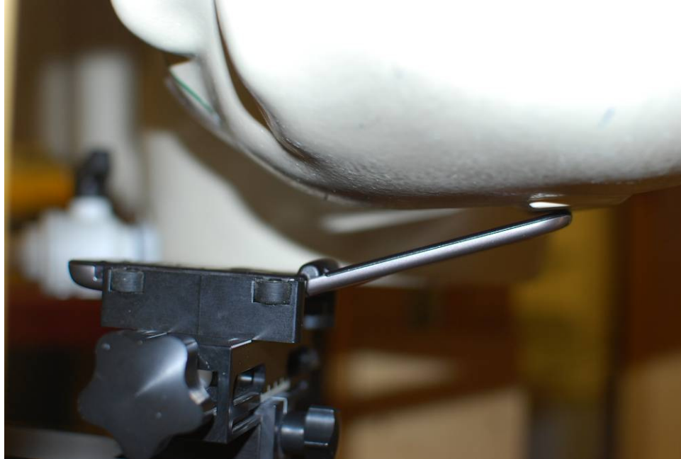
Figure 19-5 SAR Test Setup Photo 5 – Left Tilt
