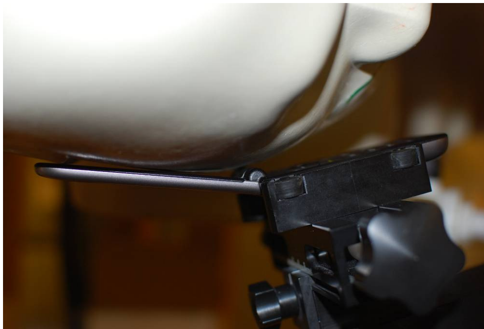
Figure 19-2 SAR Test Setup Photo 2 – Right Touch
