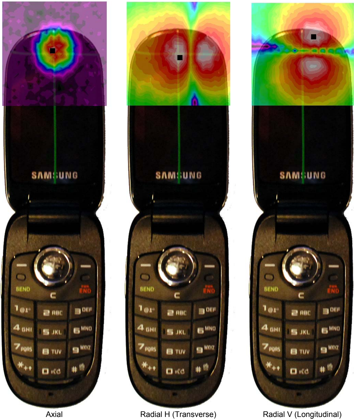
Figure 13-3 T-Coil Scan Overlay Magnetic Field Distributions
