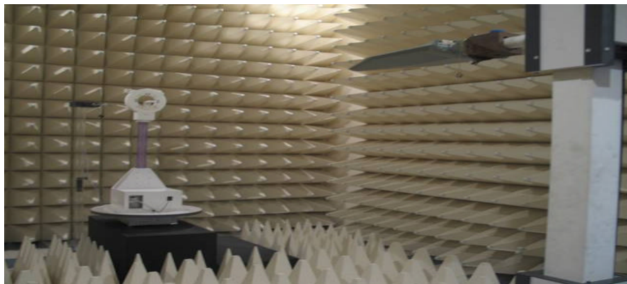
Figure2. Photograph of 3m Fully-Anechoic Chamber
