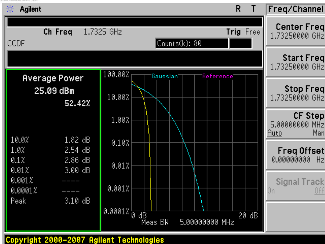
Plot 7-19. Peak-Average Ratio Plot (AWS CDMA Mode – Ch. 450)
