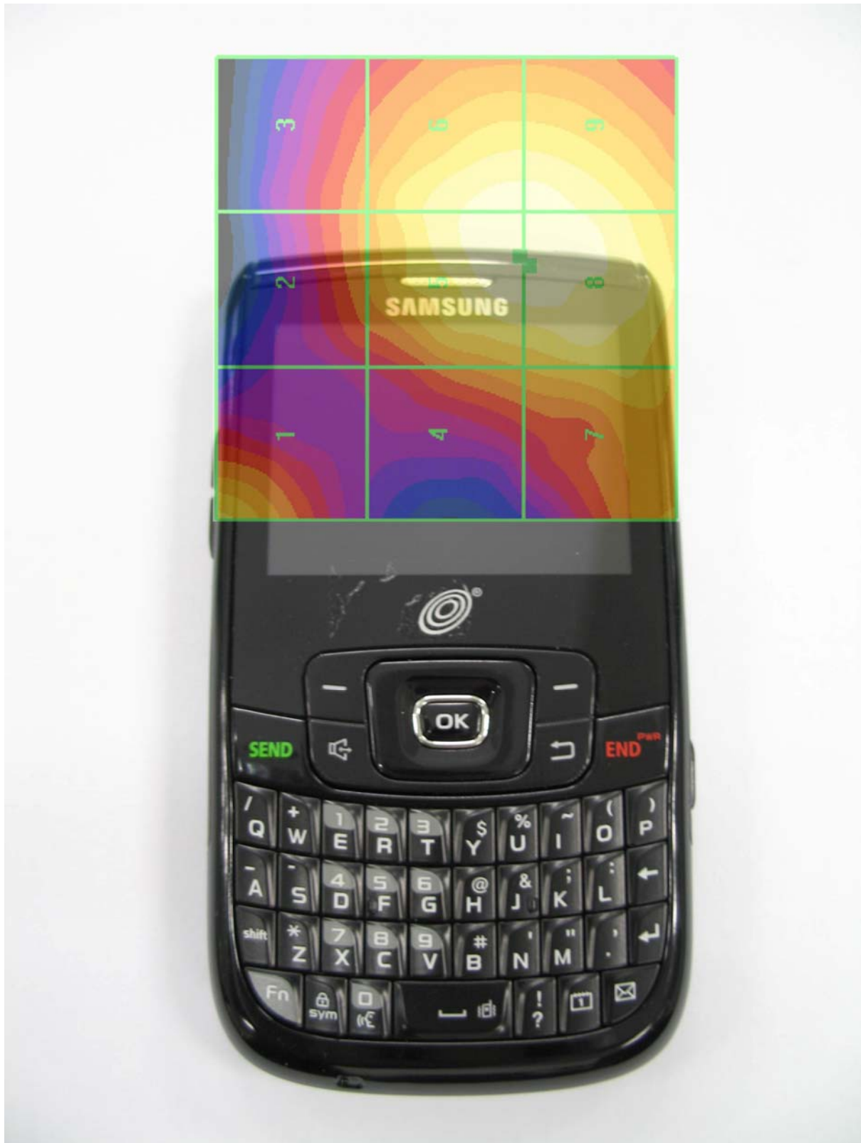
Scan overlay with actual device for PCS(H-field)
