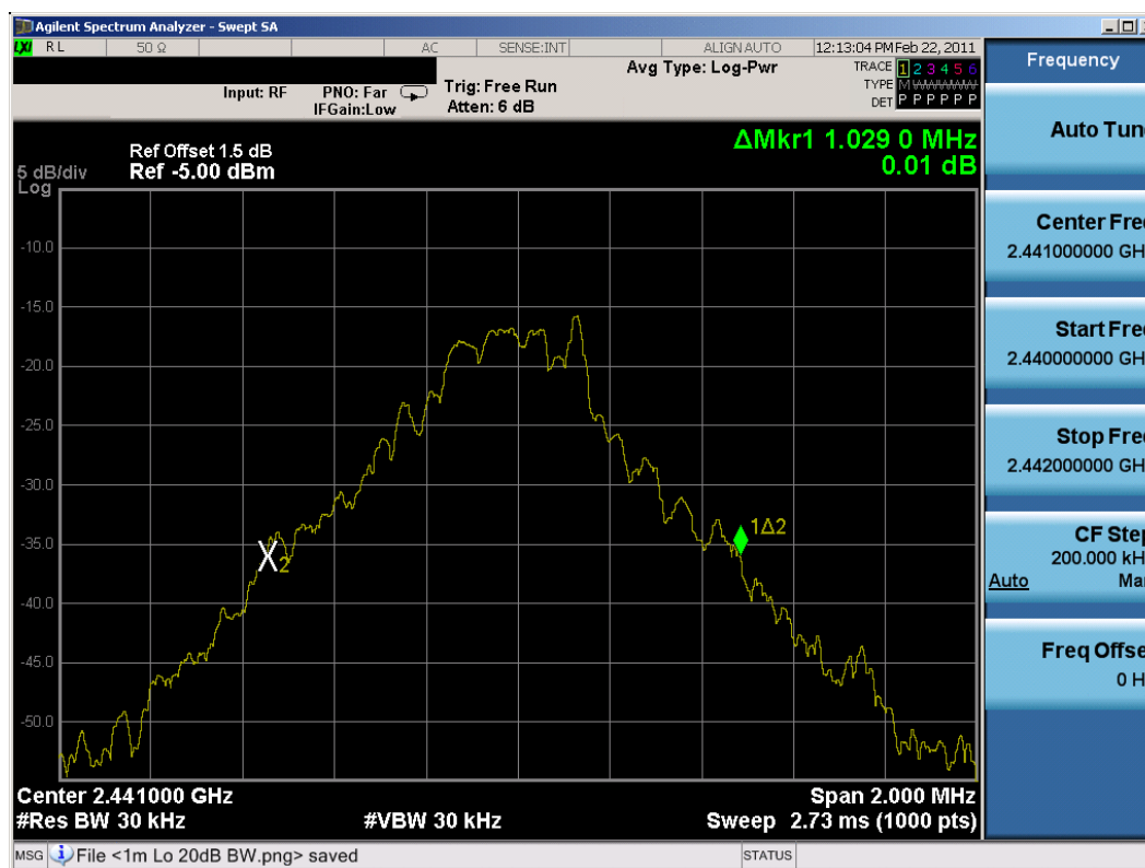
Plot 6-2. 20dB Bandwidth Plot (Bluetooth, 1Mbps – Ch. 39)
