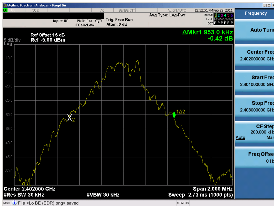
Plot 6-1. 20dB Bandwidth Plot (Bluetooth, 1Mbps – Ch. 0)
