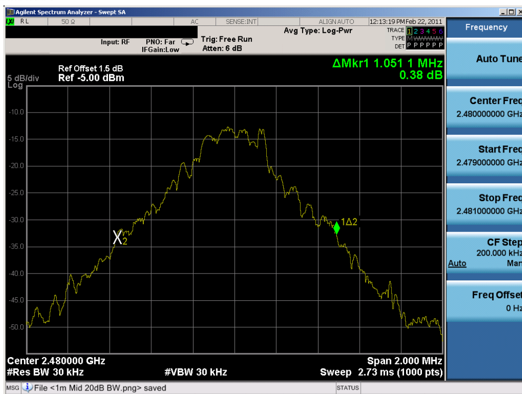
Plot 6-3. 20dB Bandwidth Plot (Bluetooth, 1Mbps – Ch. 78)
