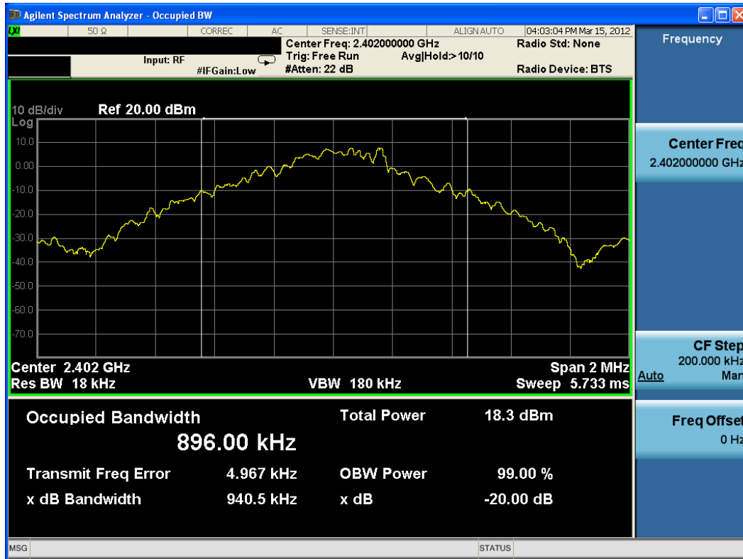
Plot 6-1. 20dB Bandwidth Plot (Bluetooth, 1Mbps – Ch. 0)
