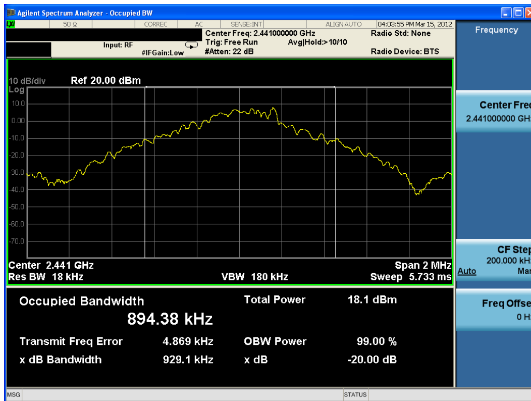
Plot 6-2. 20dB Bandwidth Plot (Bluetooth, 1Mbps – Ch. 39)
