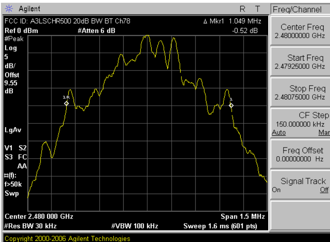
Plot 6-3. 20dB Bandwidth Plot (Bluetooth – Ch. 78)
