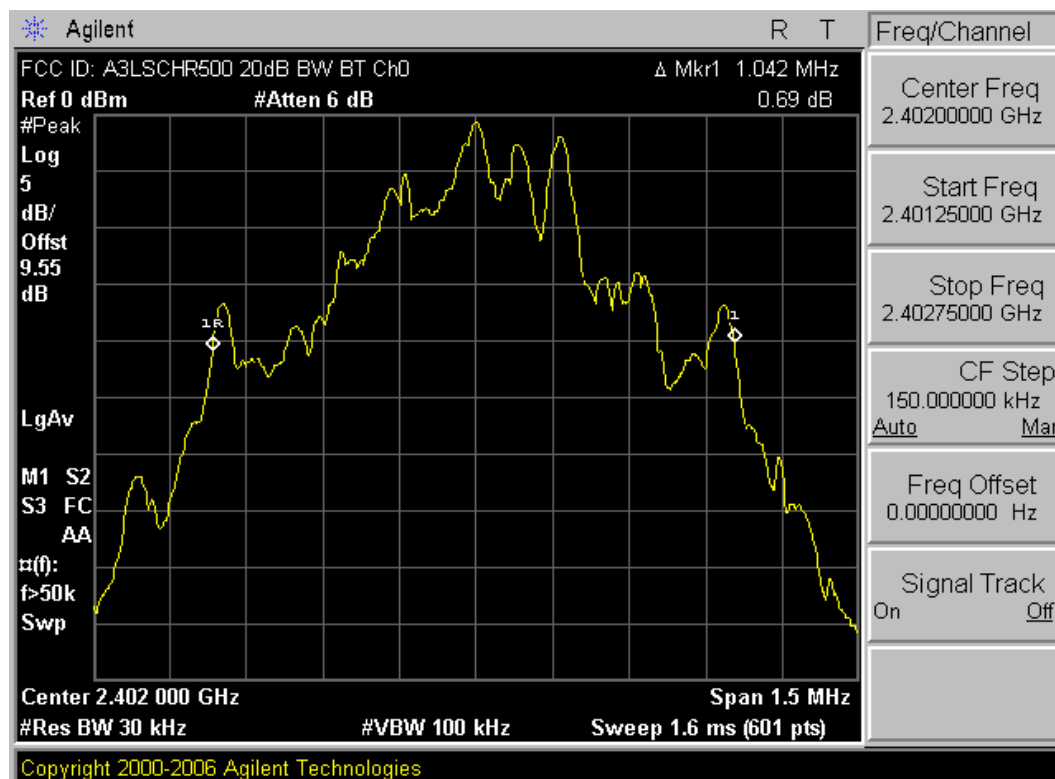
Plot 6-1. 20dB Bandwidth Plot (Bluetooth – Ch. 0)
