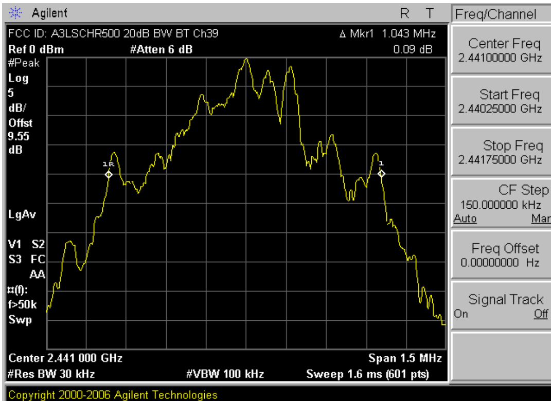
Plot 6-2. 20dB Bandwidth Plot (Bluetooth – Ch. 39)
