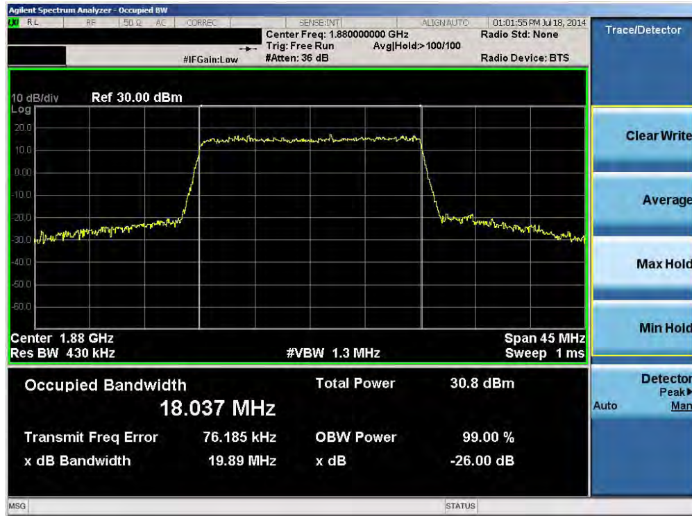
Plot 6-7. Occupied Bandwidth Plot (Band 2 – 20.0MHz QPSK – RB Size 100)
