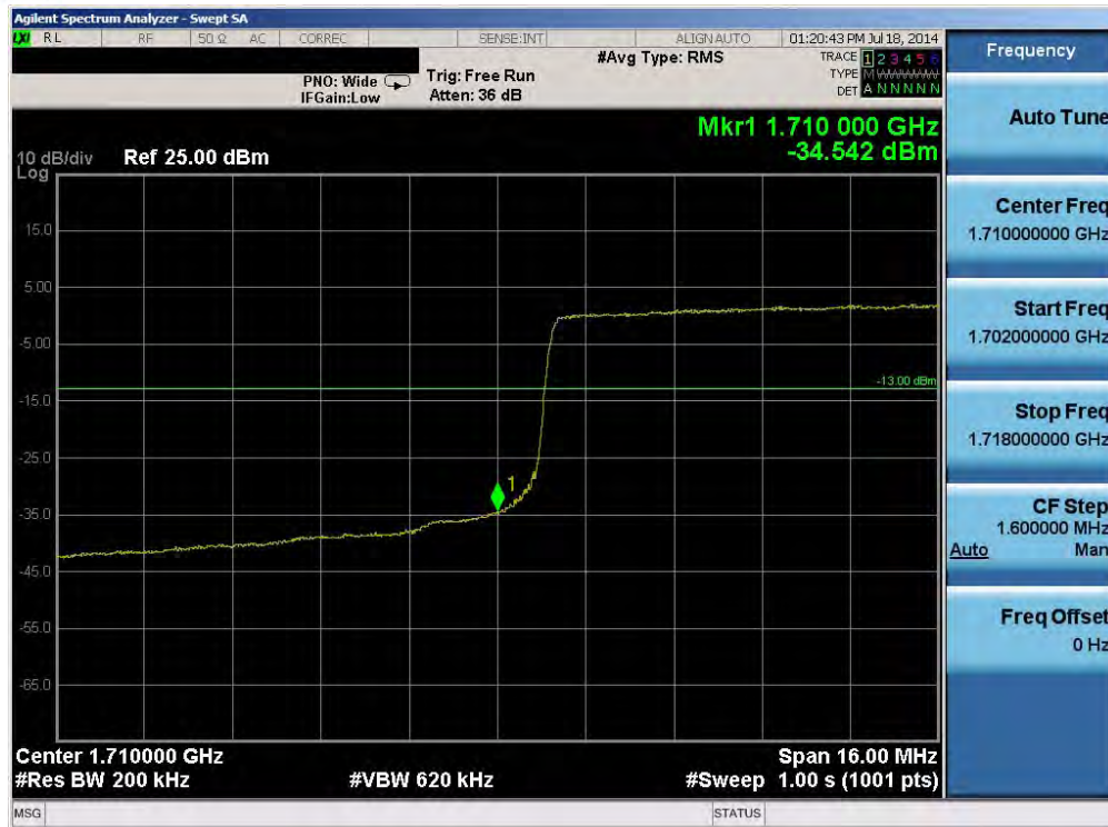
Plot 6-37. Lower Band Edge Plot (Band 4 – 20.0MHz QPSK – RB Size 100)
