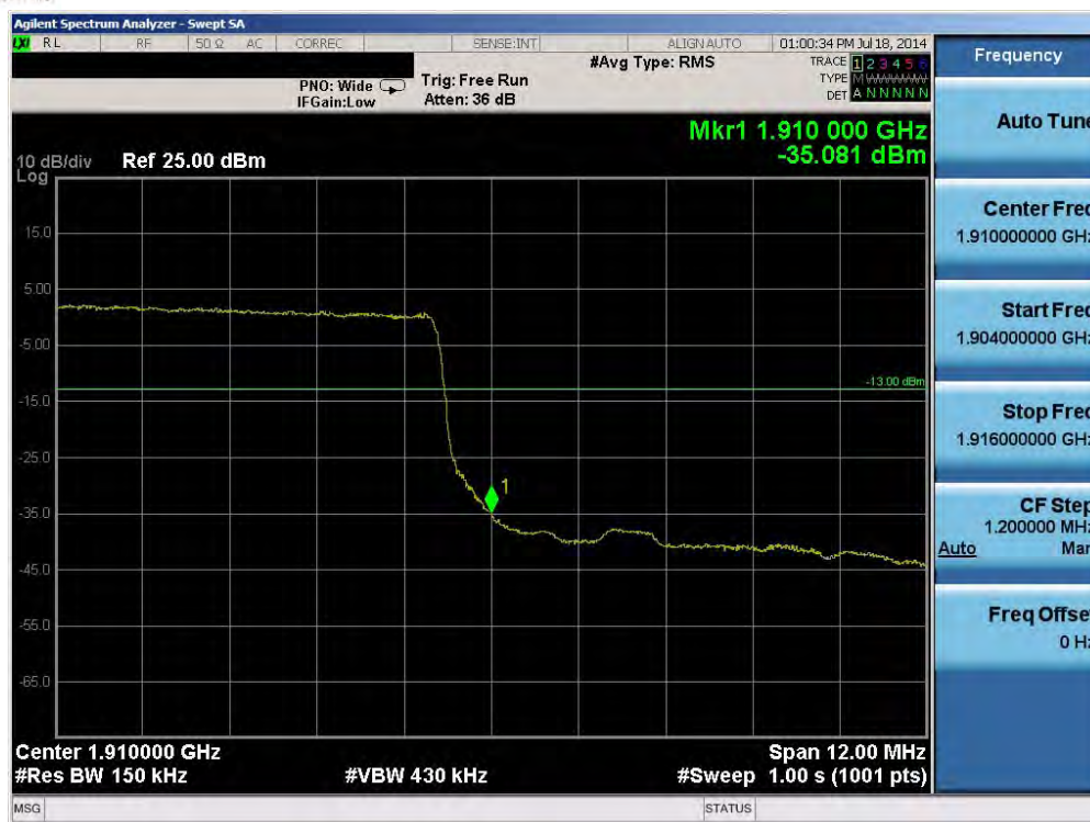
Plot 6-43. Upper Band Edge Plot (Band 2 - 15.0MHz QPSK - RB Size 75)
