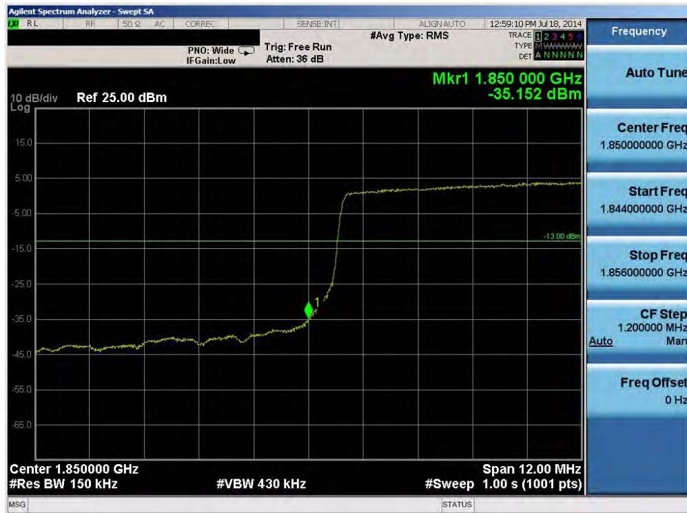
Plot 6-41. Lower Band Edge Plot (Band 2 – 15.0MHz QPSK – RB Size 75)
