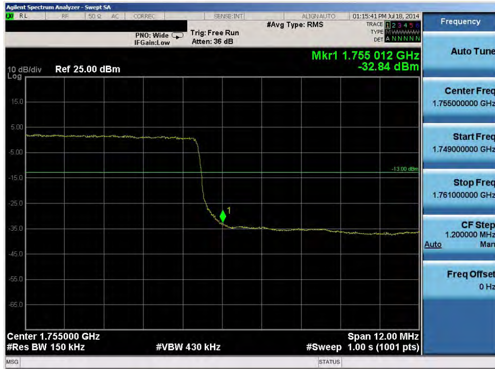
Plot 6-35. Upper Band Edge Plot (Band 4 - 15.0MHz QPSK - RB Size 75)
