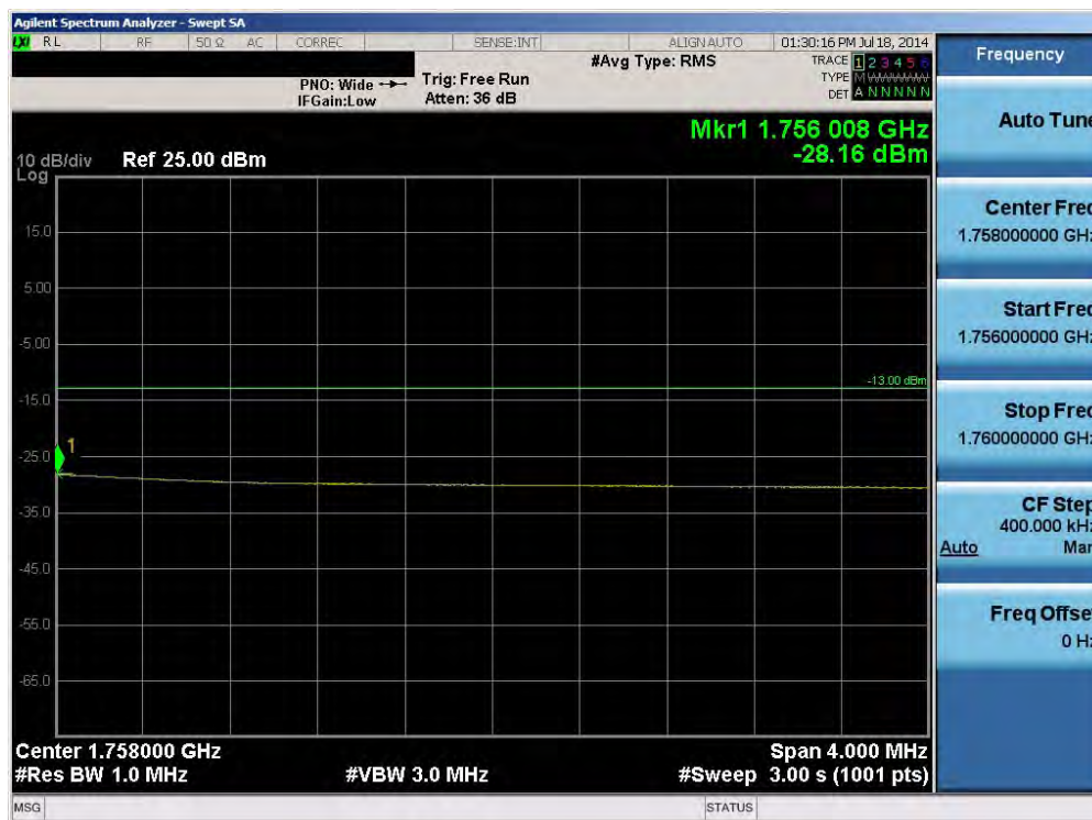
Plot 6-40. Upper Extended Band Edge Plot (Band 4 – 20.0MHz QPSK – RB Size 100)
