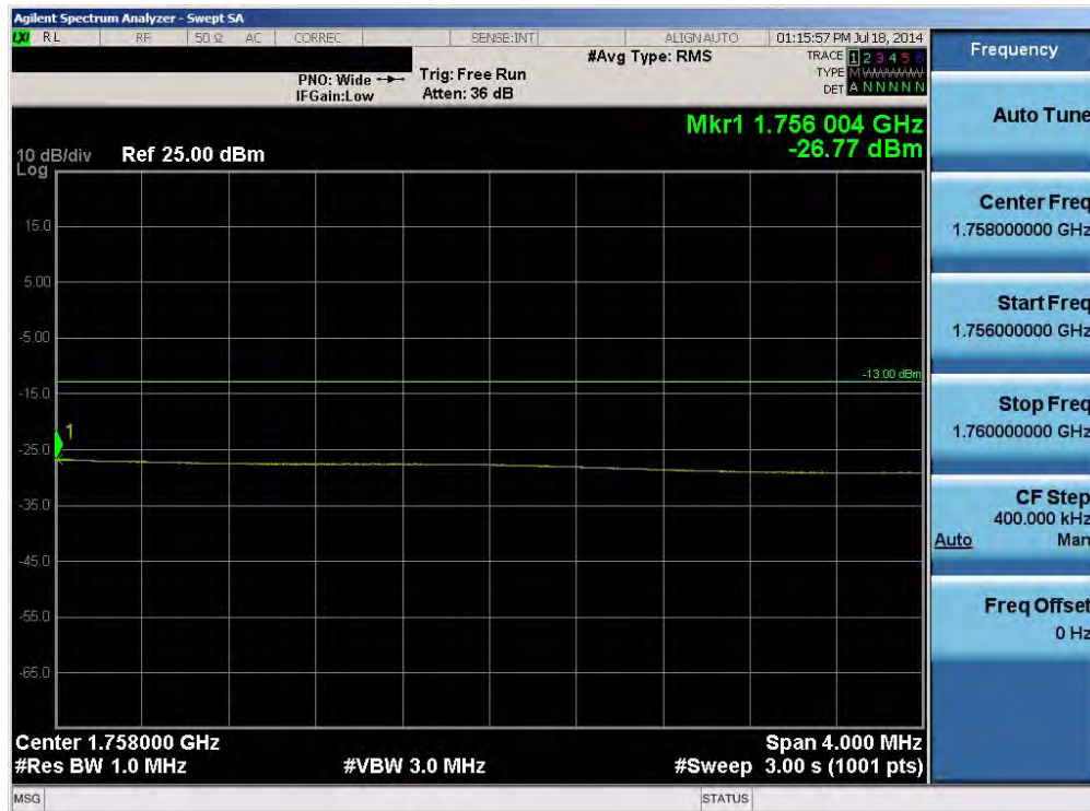
Plot 6-36. Upper Extended Band Edge Plot (Band 4 - 15.0MHz QPSK - RB Size 75)
