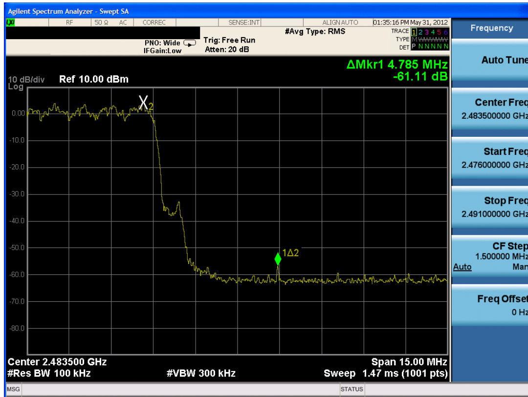
Plot 6-13. Band Edge Plot (Bluetooth with Hopping Enabled, 1Mbps)
