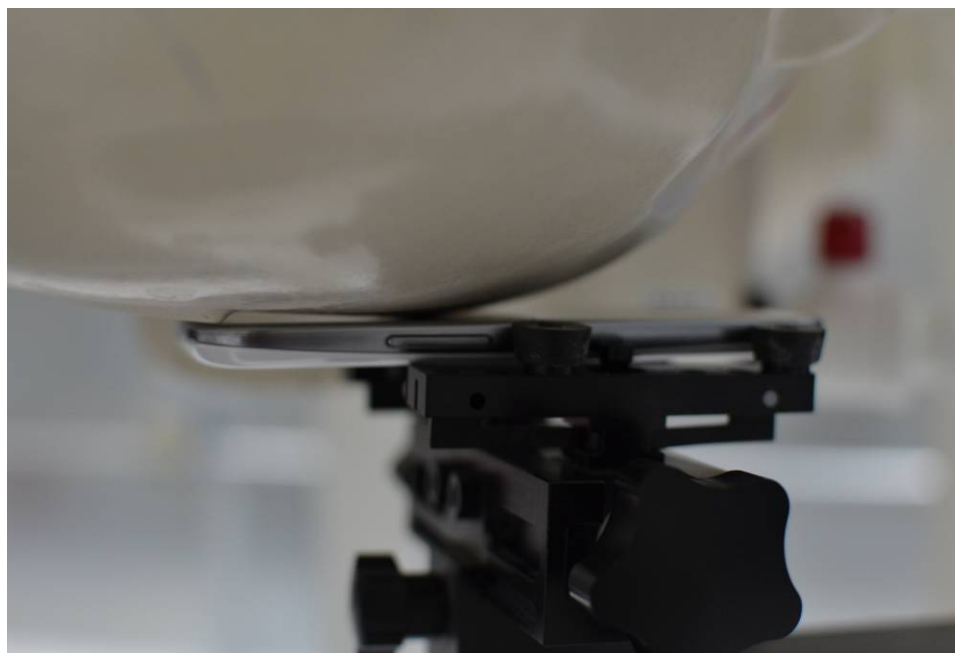
SAR Test Setup Photo 1 – Right Touch
