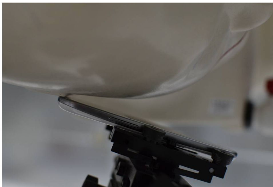
SAR Test Setup Photo 2 – Right Tilt
