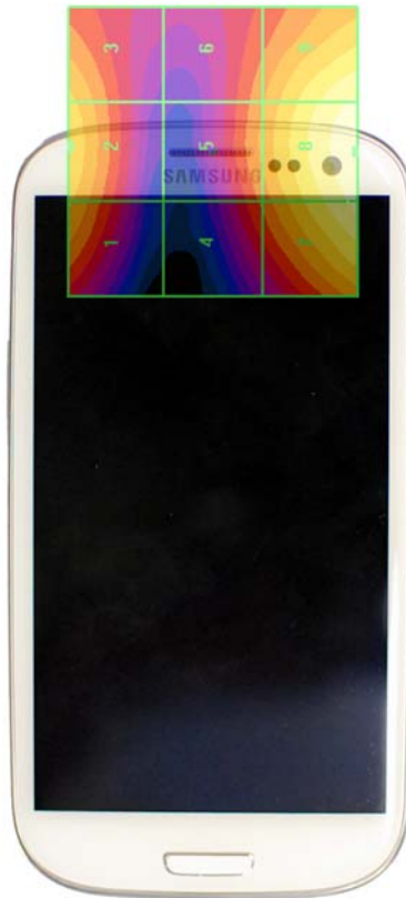
Figure 17-4 E-Field WD Scan overlay
