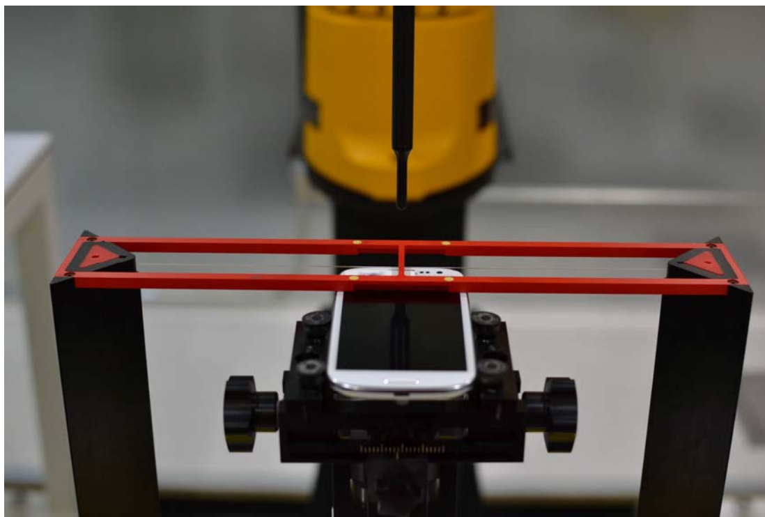
Figure 17-1 Ear Reference Point HAC Phantom Alignment
