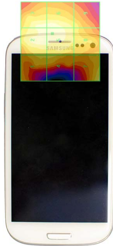
Figure 17-5 H-Field WD Scan overlay
