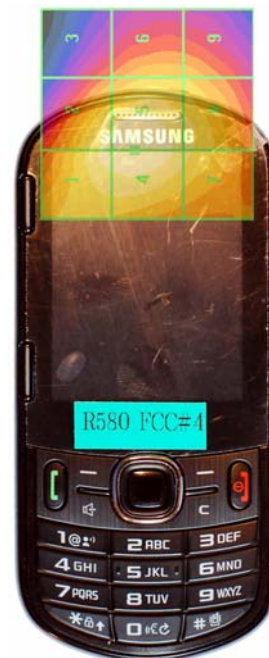
Figure 17-5 H-Field WD Scan overlay
