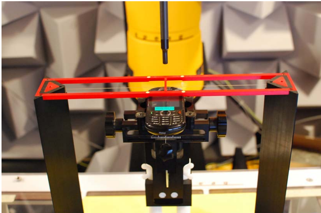
Figure 17-2 HAC Phantom Plane Alignment
