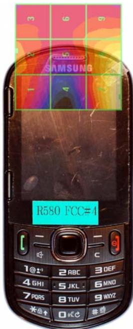
Figure 17-4 E-Field WD Scan overlay
