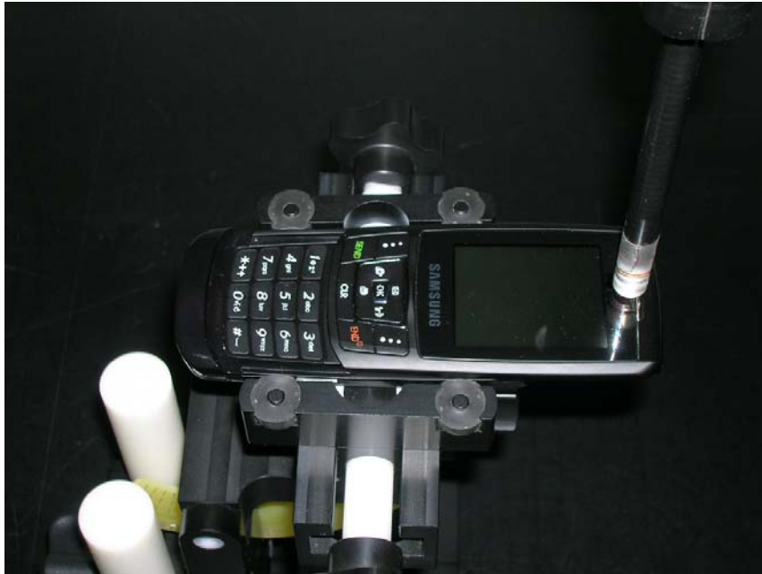
Figure 13-1 Test Setup for Wireless Device
