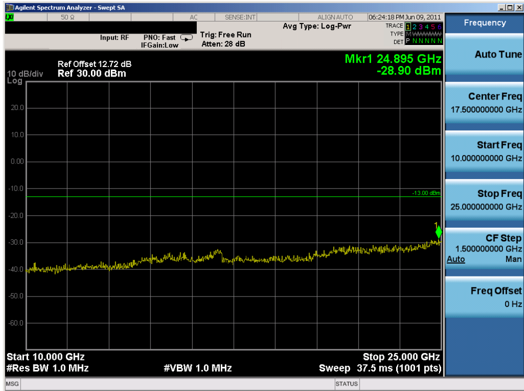
Plot 7-17. Conducted Spurious Plot (AWS CDMA Mode – Ch. 450)
