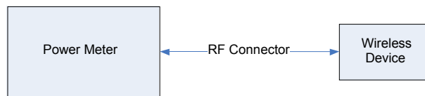
Figure 12-2 Power Measurement Setup
