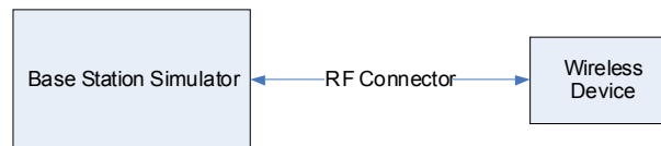
Figure 12-1 Power Measurement Setup
