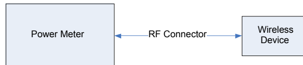
Figure 9-2 Power Measurement Setup
