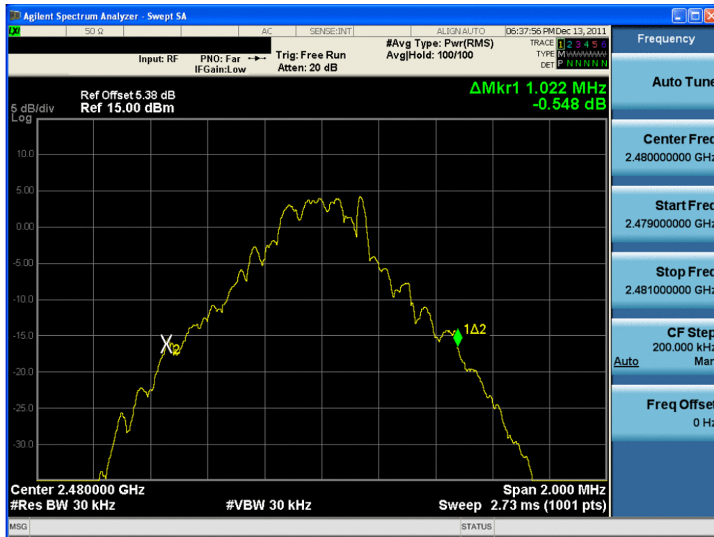
Plot 6-3. 20dB Bandwidth Plot (Bluetooth, 1Mbps – Ch. 78)
