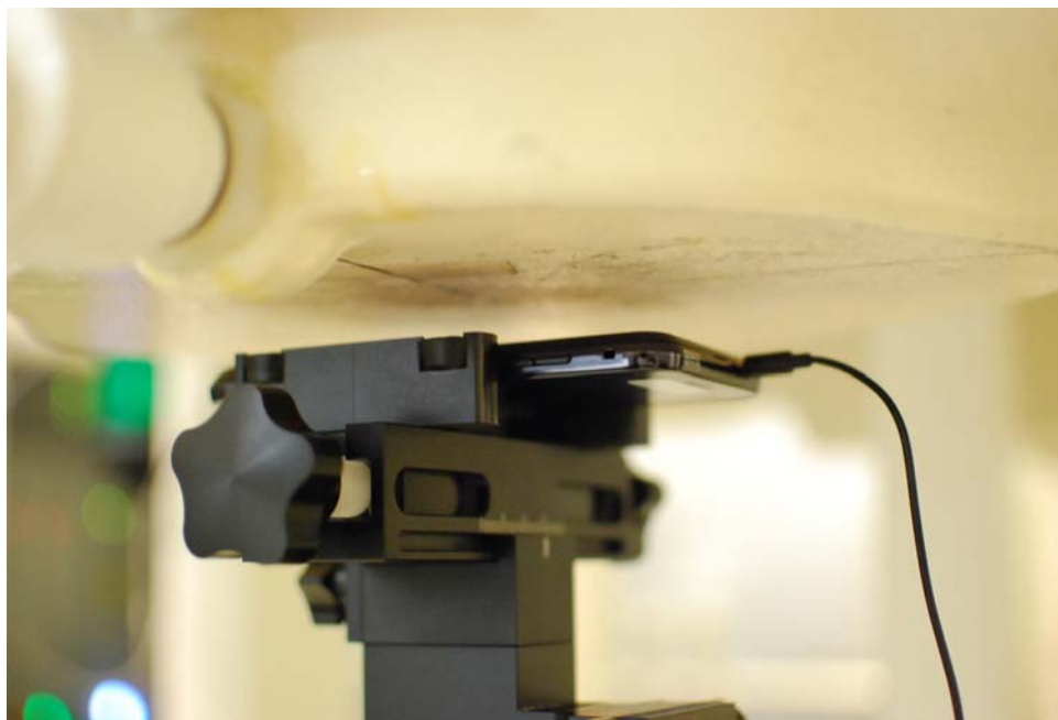
SAR Test Setup Photo 10: Body-Worn at 1.0 cm
