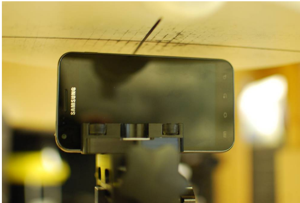
SAR Test Setup Photo 8 – Right Side at 1.0 cm
