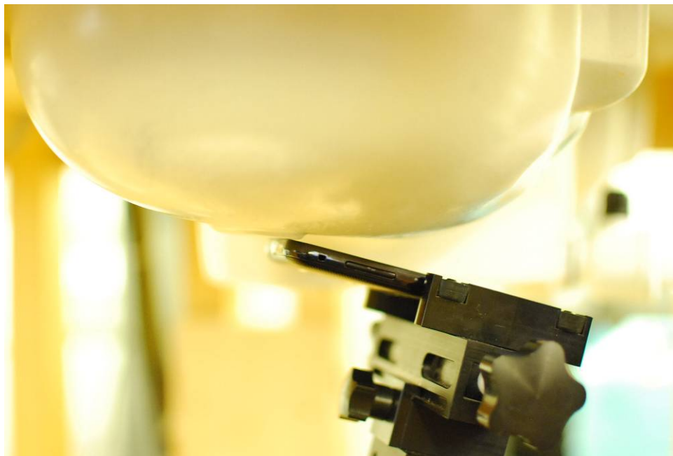
SAR Test Setup Photo 2 – Right Tilt
