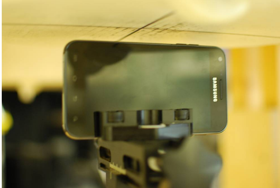
SAR Test Setup Photo 9 – Left Side at 1.0 cm
