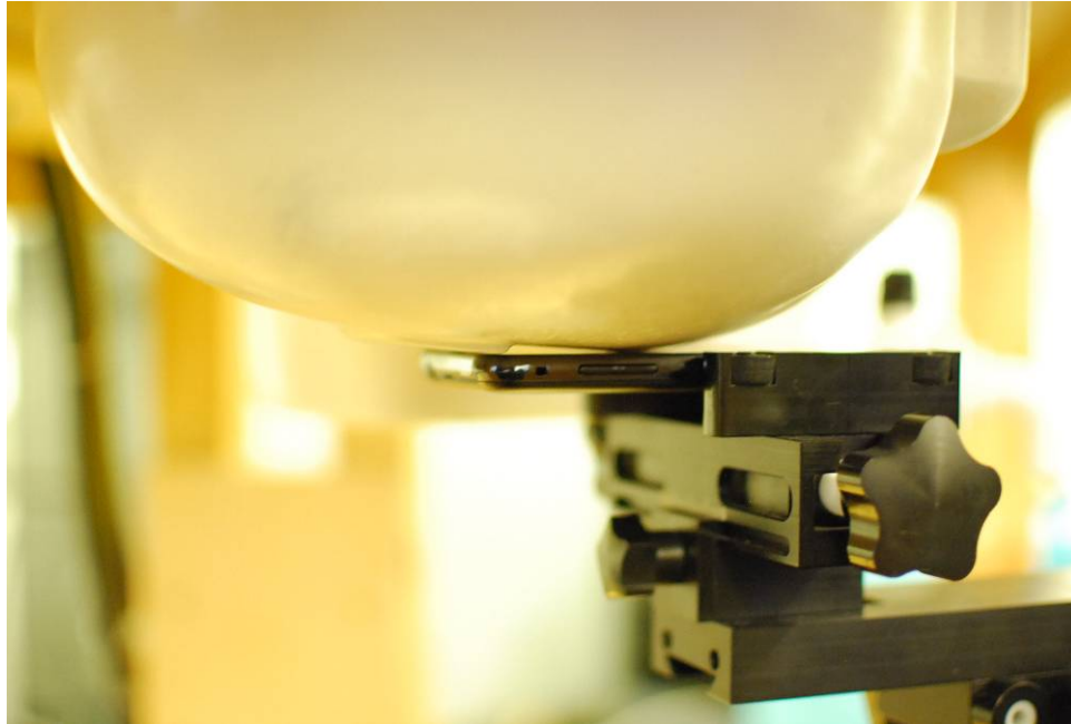
SAR Test Setup Photo 1 – Right Touch
