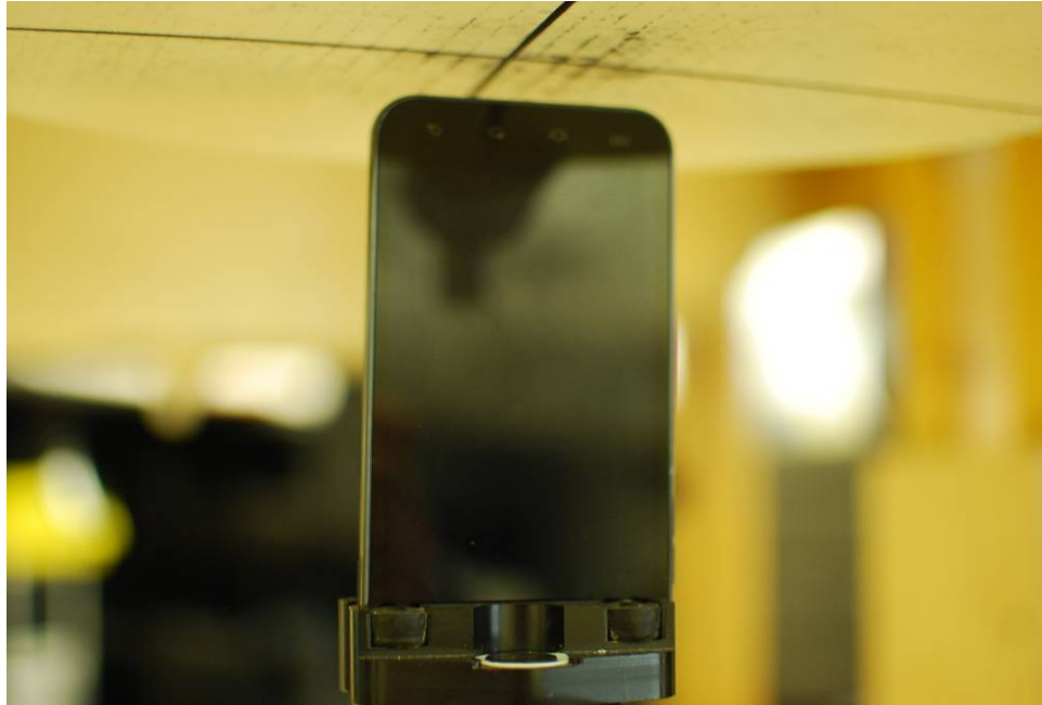
SAR Test Setup Photo 7 – Bottom at 1.0 cm
