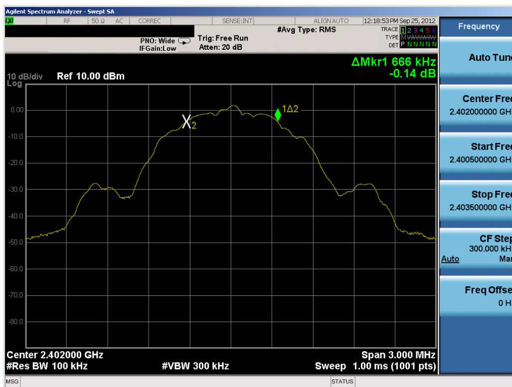
Plot 6-1. 6dB Bandwidth Plot (Bluetooth (LE) – Ch. 0)
