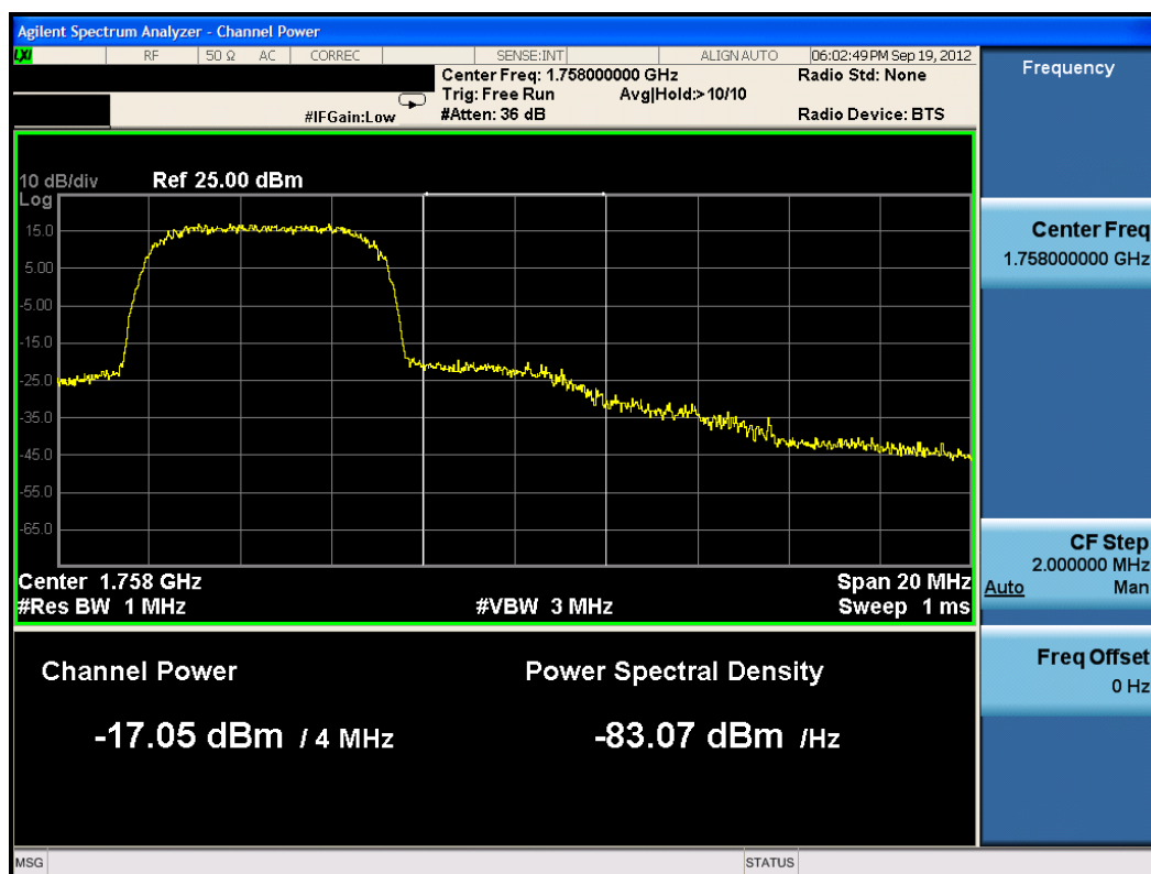
Plot 9-17. Upper Extended Band Edge Plot (5MHz QPSK– RB Size 25)
