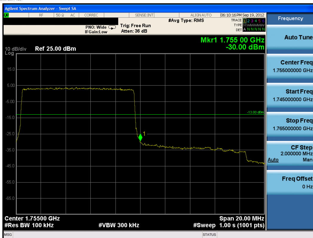
Plot 9-16. Upper Band Edge Plot (10MHz QPSK – RB Size 50)
