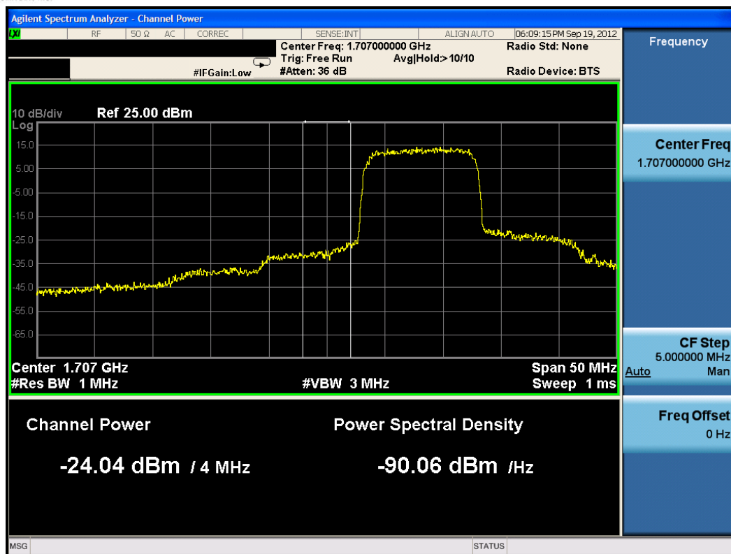
Plot 9-4. Lower Extended Band Edge Plot (10MHz QPSK– RB Size 50)
