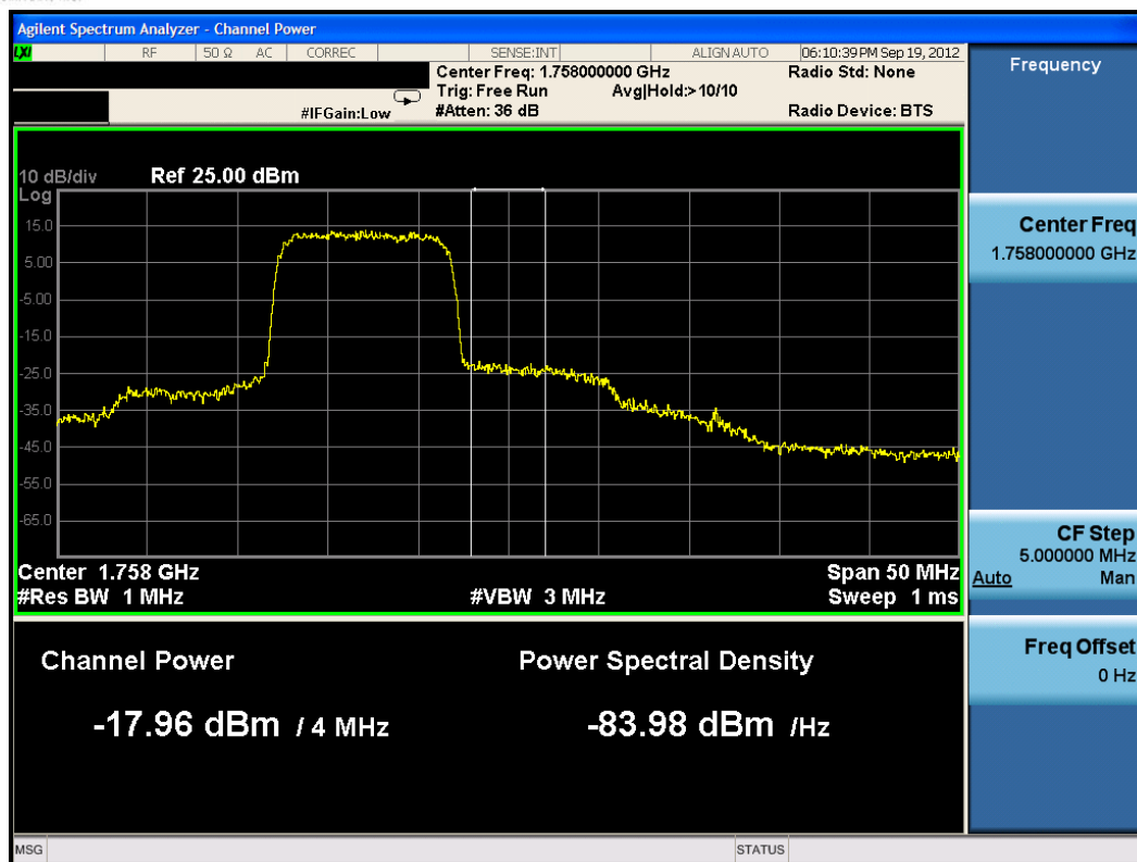
Plot 9-18. Upper Extended Band Edge Plot (10MHz QPSK– RB Size 50)
