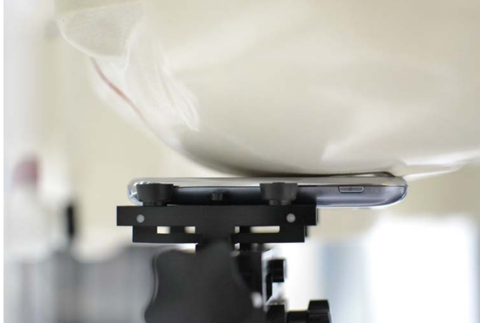
SAR Test Setup Photo 3: Left Touch
