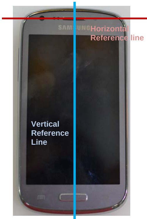
SAR Test Setup Photo 9: DUT reference lines
