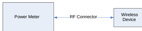
Figure 9-2 Power Measurement Setup
