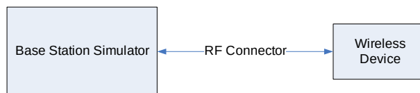
Figure 9-1 Power Measurement Setup
