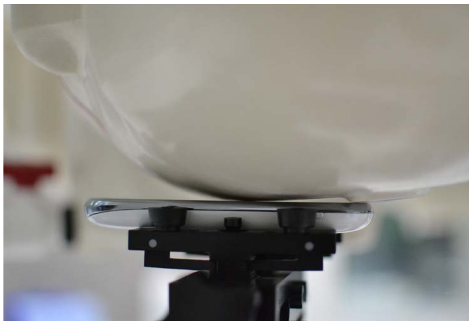
SAR Test Setup Photo 3 – Left Cheek
