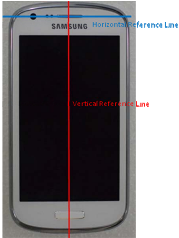
SAR Test Setup Photo 11 – DUT Horizontal and Vertical Reference Lines
