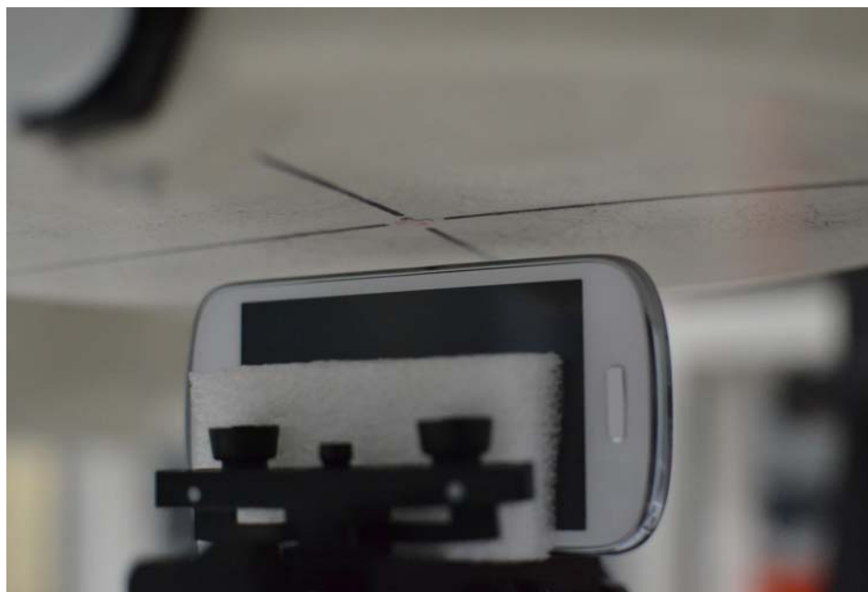
SAR Test Setup Photo 7 – Right Edge at 1.0 cm
