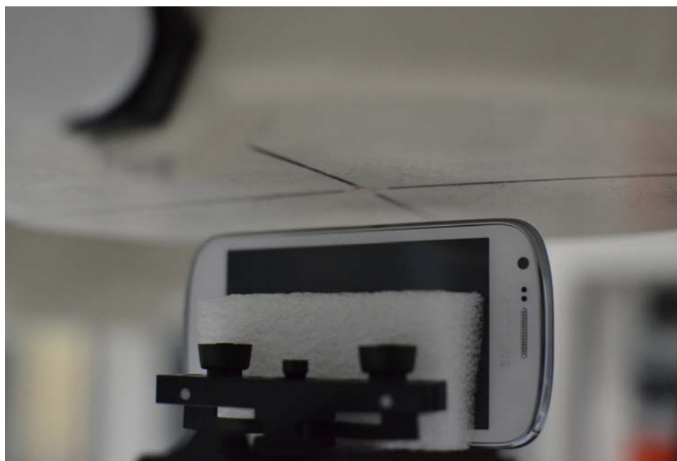
SAR Test Setup Photo 8 – Left Edge at 1.0 cm
