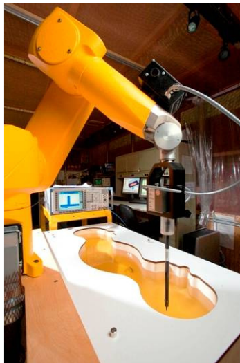
Figure 3-2 DASY4 SAR Measurement System
