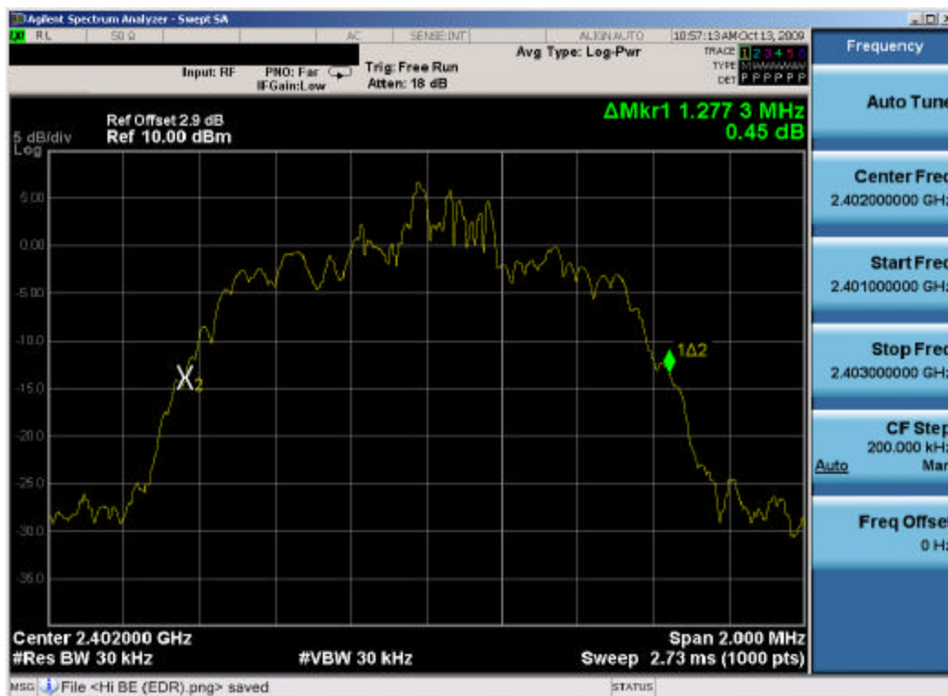
Plot 6-1. 20dB Bandwidth Plot (Bluetooth 2.0 with Enhanced Data Rates – Ch. 0)
