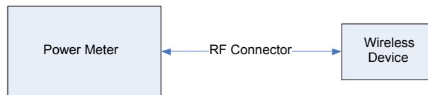
Figure 13-1 Power Measurement Setup
