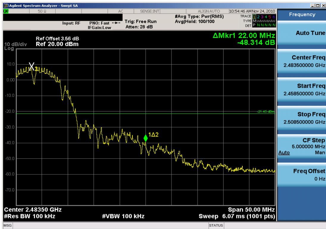
Plot 6-20. Band Edge Plot (802.11b – Ch. 11)
