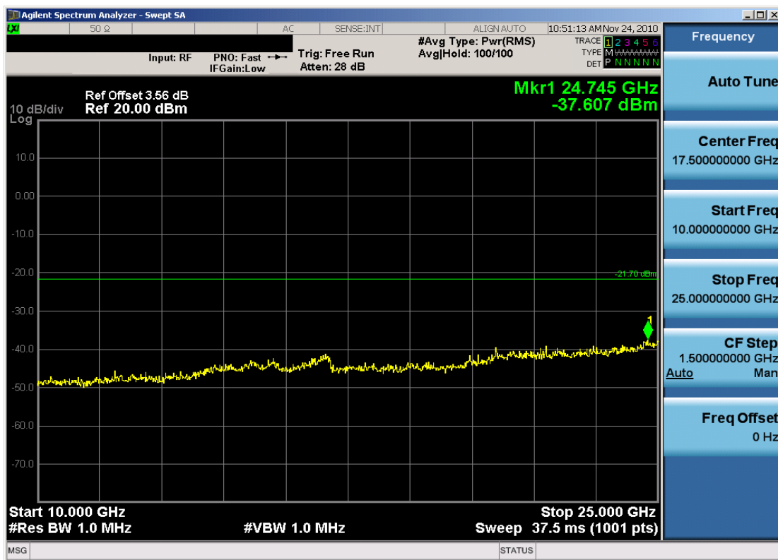
Plot 6-28. Conducted Spurious Plot (802.11b – Ch. 6)
