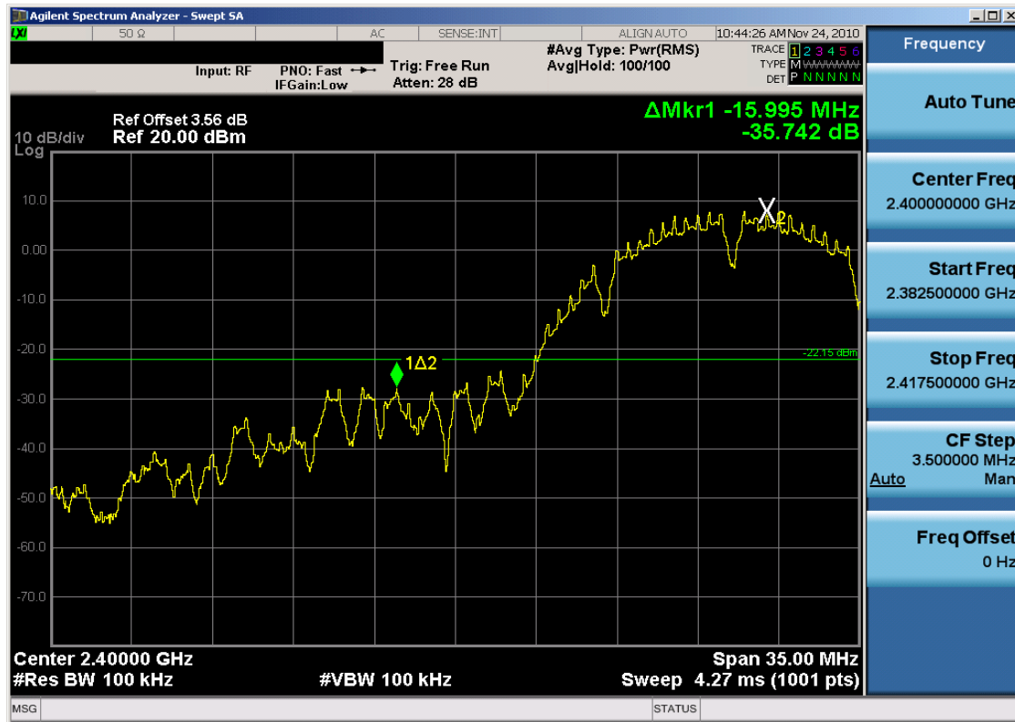
Plot 6-19. Band Edge Plot (802.11b – Ch. 1)
