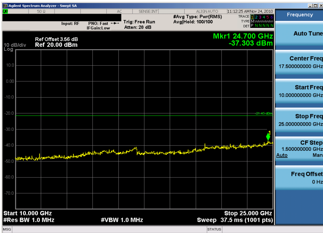
Plot 6-30. Conducted Spurious Plot (802.11b – Ch. 11)
