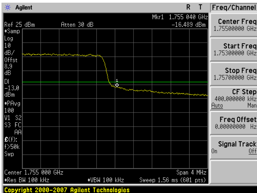
Plot 7-36. Band Edge Plot (5MHz BW, QPSK, AWS Band – High Channel)
