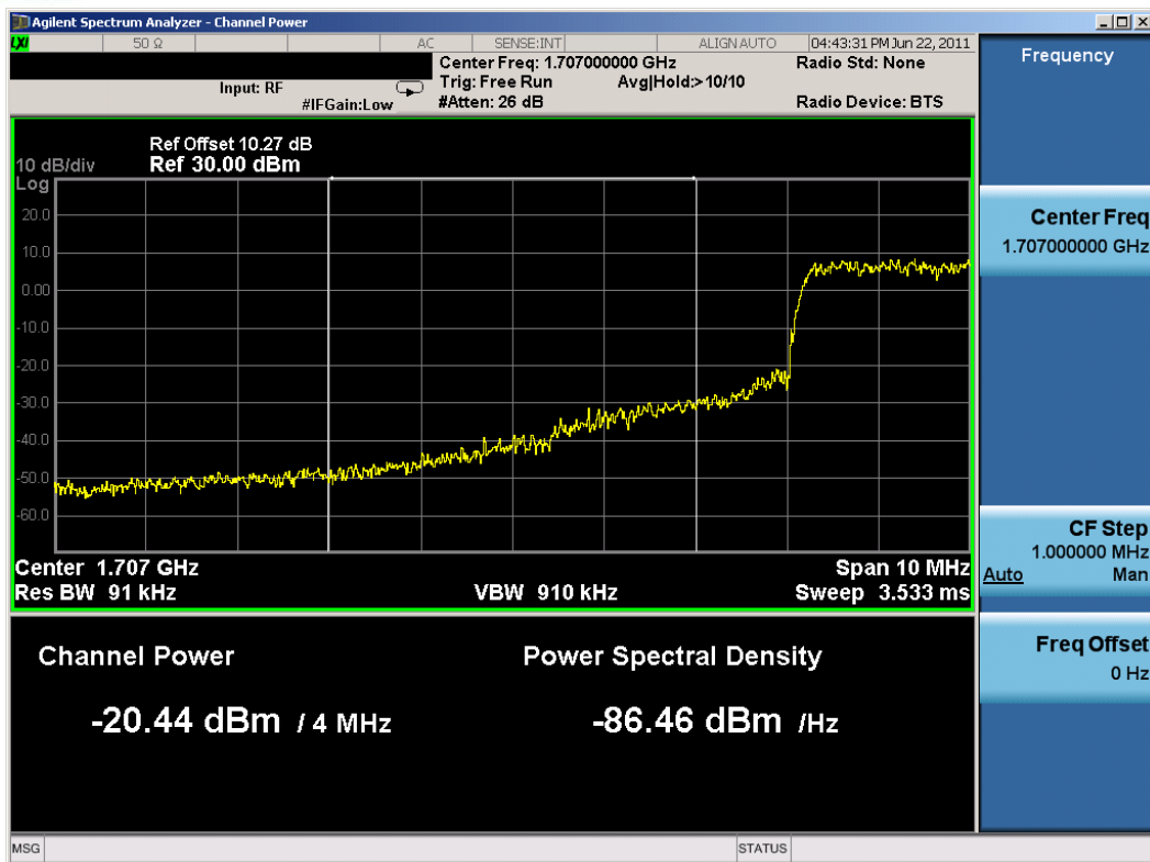
Plot 7-18. 4MHz Span Plot (3MHz BW, QPSK, AWS Band – Low Channel)
